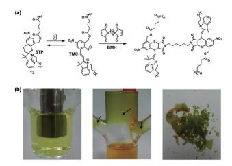
Fig. 14 (a) Crosslinking pathway based on the STP system. (b) The sonication apparatus before (left) and after (middle) 20 min of sonication, and the material peeled from the walls of the sonication cell (right). Reproduced with permission.<sup>52</sup> Copyright 2016, John Wiley and Son.
