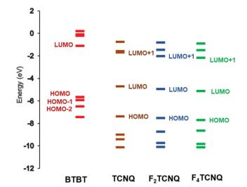
Fig. 4 Energy levels of the BTBT, TCNQ, F2TCNQ, and F4TCNQ molecules, as calculated at the B3LYP/6-31G(d,p) level.
