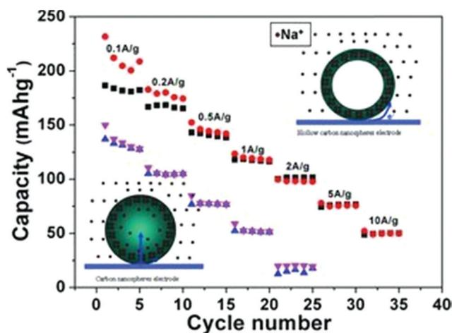
**Fig. 17** Schemes of the electrochemical reaction process and realistic rate performance of HCNs and solid carbon spheres. Reproduced with permission.<sup>55</sup> Copyright 2012, Wiley-VCH.
