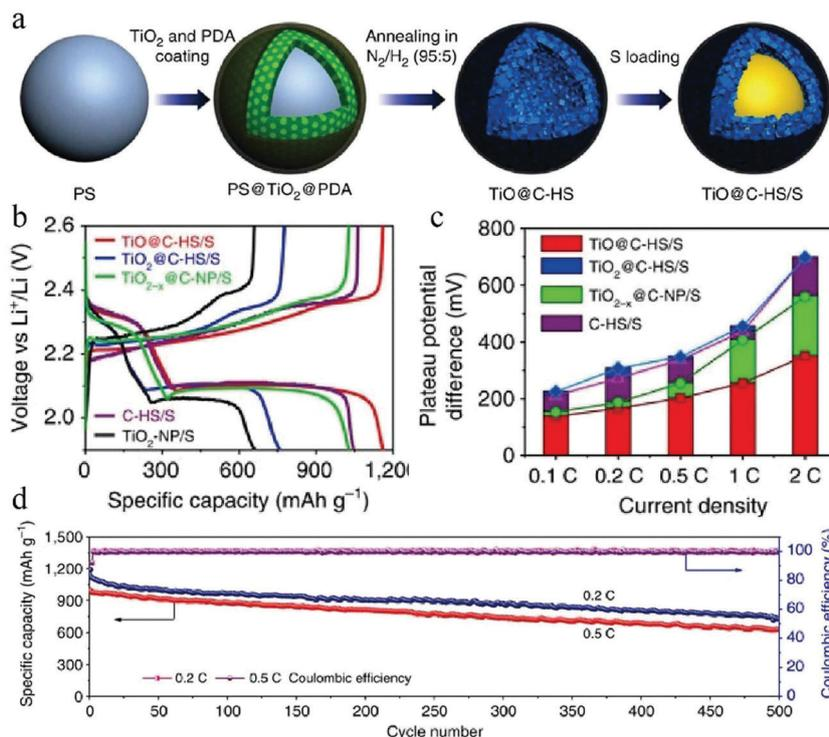
**Fig. 16** (a) Schematic illustration of the synthesis process of the TiO@C-HS/S composite. (b) Second-cycle galvanostatic charge/discharge voltage profiles at 0.1C. (c) Potential differences between the charge and discharge plateaus at various current densities of the electrodes. (d) Prolonged cycling life and coulombic efficiency of the TiO@C-HS/S electrode at 0.2 and 0.5C. Reproduced with permission.<sup>4a</sup> Copyright 2016, Nature.
