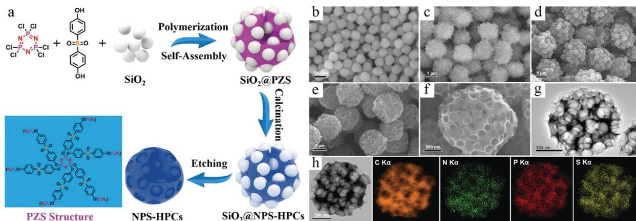
Fig. 4 (a) Schematic illustration for preparing nitrogen, phosphorus, and sulfur codoped hierarchical porous carbon spheres (NPS-HPCs). SEM images of (b) SiO<sub>2</sub> NPs, (c) self-assembly of SiO<sub>2</sub>@PZS, (d) SiO<sub>2</sub>@NPS-HPCs, and (e and f) NPS-HPCs. (g) TEM image of NPS-HPCs. (h) Energy-dispersive X-ray spectroscopy (EDS) mapping images of NPS-HPCs. Reproduced with permission.<sup>27</sup> Copyright 2018, American Chemical Society.
