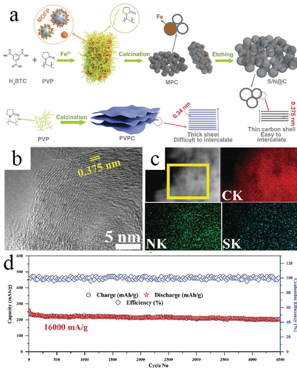
**Fig. 18** (a) Schematic representation of S/N@C synthesis. (b) HRTEM and (c) HAADF analysis of S/N@C. (d) Cycling performance at a current density of  $16\,000\text{ mA g}^{-1}$ . Reproduced with permission.<sup>57</sup> Copyright 2019, Wiley-VCH.
