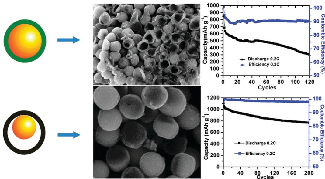
Fig. 14 Schematic comparison of the S-PANI core-shell and yolk-shell SEM images after running five cycles in cells and long-term cycling performance. Reproduced with permission.<sup>25</sup> Copyright 2013, American Chemical Society.
