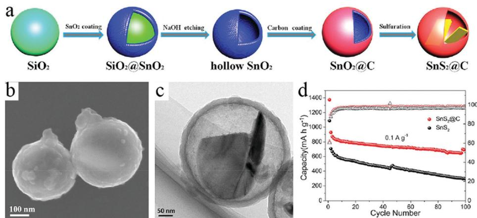
Fig. 19 (a) Schematic of the formation process of SnS<sub>2</sub>@C. (b) SEM and (c) TEM images of the as-prepared SnS<sub>2</sub>@C. (d) Cycling performance of SnS<sub>2</sub>@C electrode at current densities of 0.1 A g<sup>-1</sup>. Reproduced with permission.<sup>61</sup> Copyright 2018, Elsevier.
