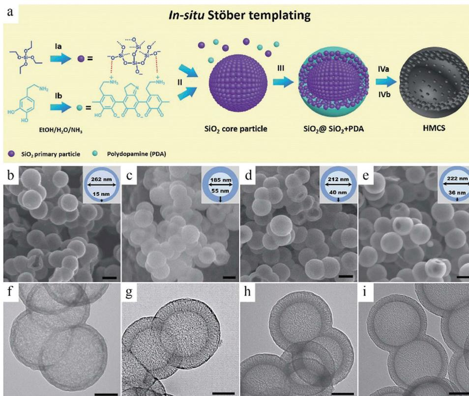
Fig. 2 (a) Schematic illustration of the *in situ* Stober templating of HMCS. (b–e) SEM and (f–i) TEM images of HMCSs with different core–shell sizes for different concentrations and addition times of dopamine. Reproduced with permission.<sup>24a</sup> Copyright 2016, Royal Society of Chemistry.
