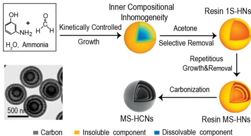
Fig. 10 Schematic of the synthesis route for hollow 3-AF structures. Reproduced with permission.<sup>35</sup> Copyright 2017, American Chemical Society.
