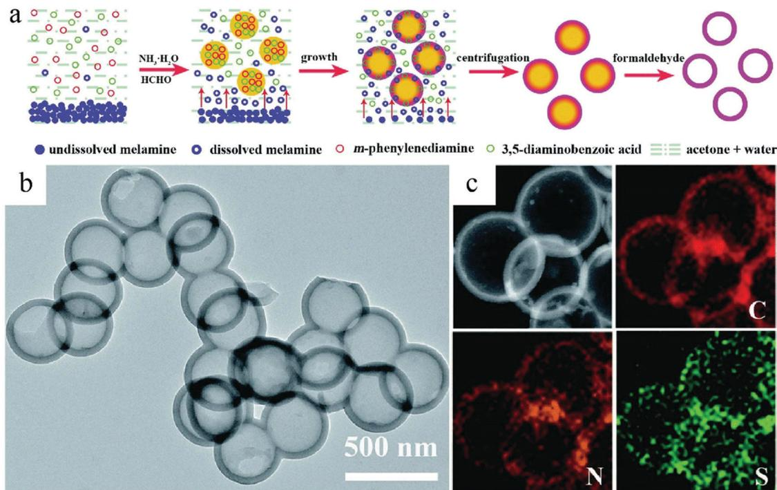
Fig. 12 (a) Illustration of the hollow polymer sphere (HPS) synthesis process. (b) TEM images of HPS and (c) the corresponding elemental mappings. Reproduced with permission.<sup>39</sup> Copyright 2020, Royal Society of Chemistry.
