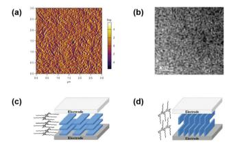
(a) AFM phase image and (b) TEM image of a typical BHJ blend film. Reproduced with permission.<sup>73</sup> Copyright 2020, American Chemical Society. Schematic illustrations of (c) face-on and (d) edge-on packing mode of active layer materials. Reproduced with permission.<sup>70</sup> Copyright 2016, American Chemical Society.
