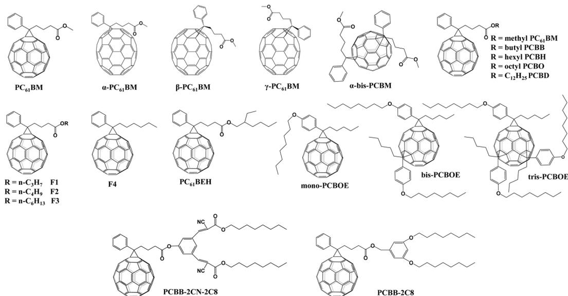
Fig. 2 Molecular structures of PC<sub>61</sub>BM and PC<sub>61</sub>BM-based fullerene derivatives applied in PSCs.
