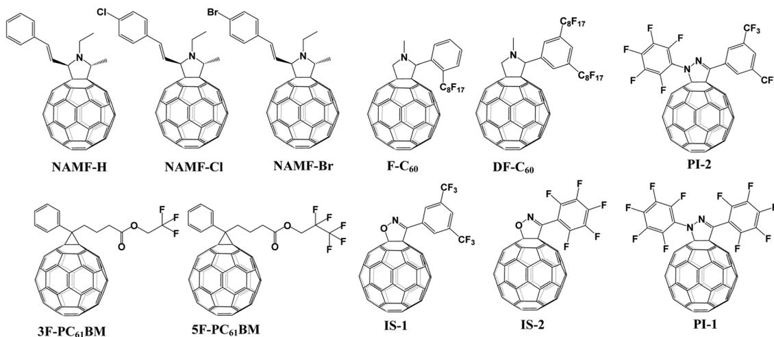
Fig. 12 Molecular structures of halogen functionalized fullerene derivatives applied in PSCs.
