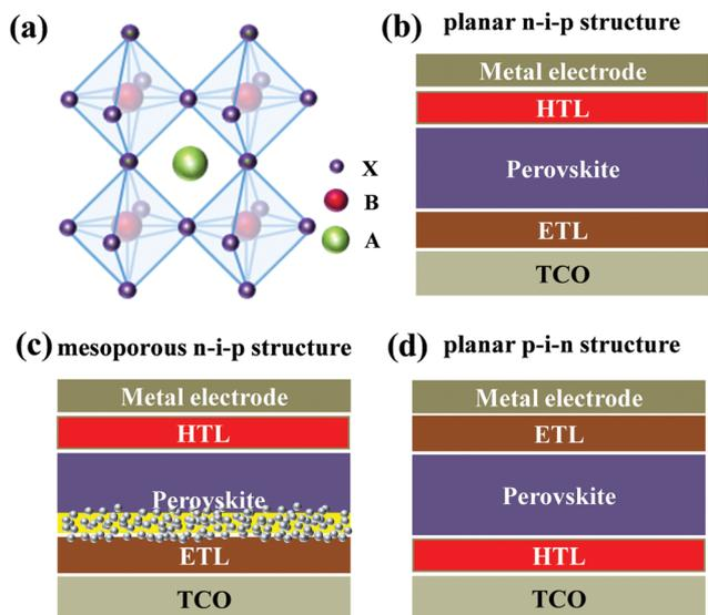
**Fig. 1** (a) Crystal structure of ABX<sub>3</sub> perovskite light-absorbing materials. The common device architectures of (b) planar n-i-p structures, (c) mesoporous n-i-p structures, and (d) planar p-i-n structures. TCO refers to transparent conductive oxide.
