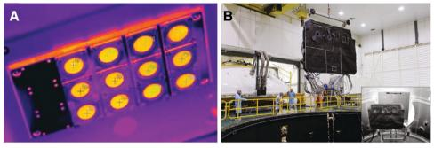
Fig. 18 Biosafety materials for aerospace safety. (A) SolarBlack material samples during testing in the Synergist Temperature Accelerated Testing (STAR) facility in the ESA/ESTEC center. (B) Solar orbiter heatshield based on SolarBlack technology. Reproduced with permission from ref. 205. Copyright 2015, Elsevier.
