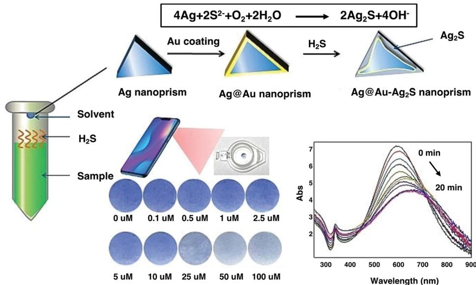
Fig. 17 Biosafety materials for food safety. Schematic illustration of the  $\text{H}_2\text{S}$  sensing mechanism based on the Ag@Au core-shell nanoprobe. Reproduced with permission from ref. 204. Copyright 2019, American Chemical Society.
