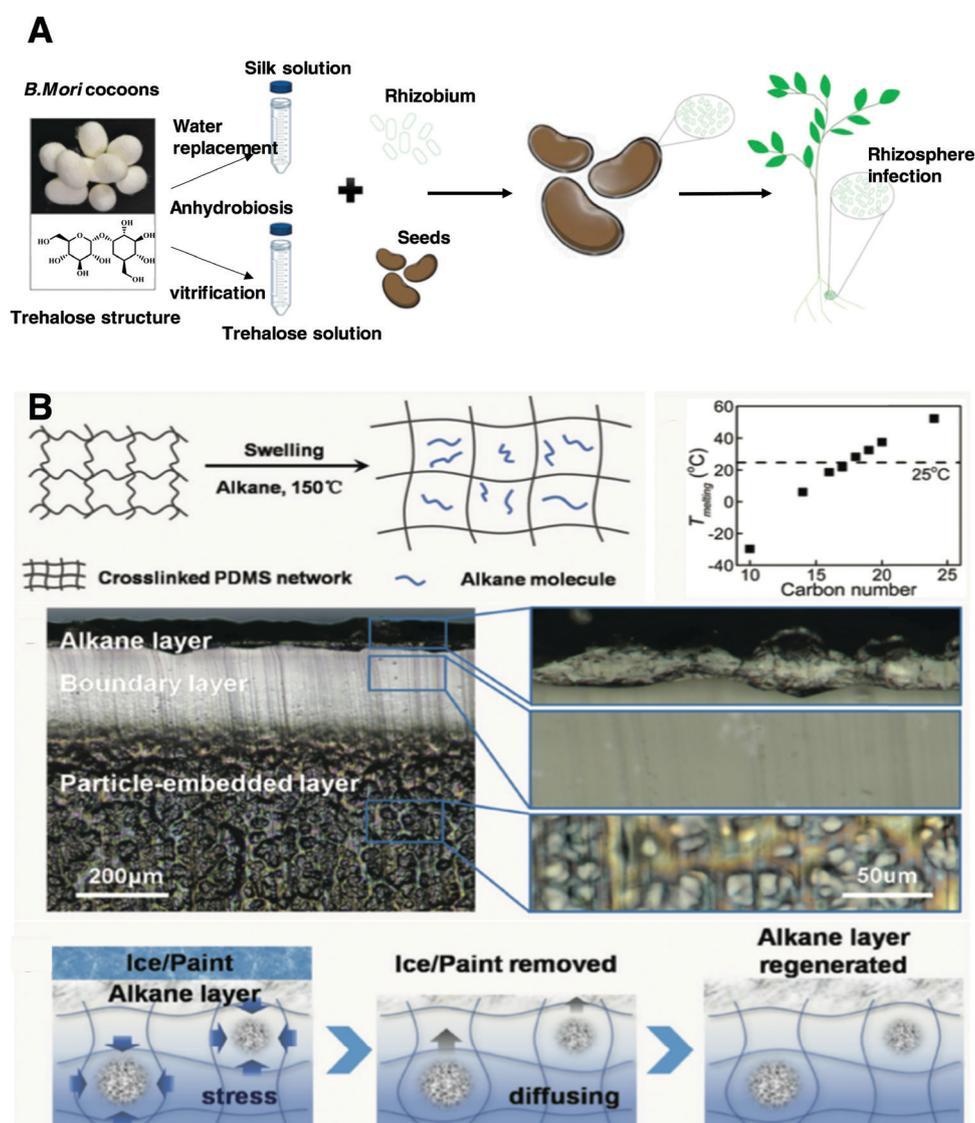
**Fig. 11** Biosafety materials for the protection and preservation of biological resources. (A) Biosafety materials based on silk fibroin and trehalose for seed coating, which can boost germination and mitigate abiotic stress. Reproduced with permission from ref. 158. Copyright 2019, National Academy of Sciences. (B) Principle of the solid organogel material to cryopreserve biological resources. Reproduced with permission from ref. 164. Copyright 2017, Wiley-VCH.
