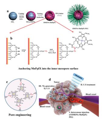
Fig. 4 A schematic diagram of how MnPpIX was covalently conjugated onto mesopore silica nanoparticles and the in vivo antitumor effect of SDT. Reproduced with permission ref. 61
