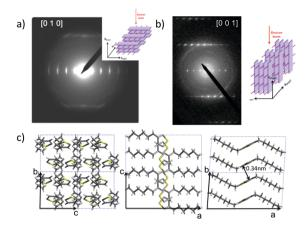
Form II. Monoclinic (P2<sub>1</sub>/c) a= 1.29nm, b = 0.94nm, c= 0.78nm  $\alpha$ =  $\beta$  = 90 deg,  $\gamma$  = 68.4 deg.
