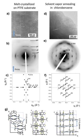
Fig. 8 Bright field images (a and d), experimental ED patterns (b and e) and calculated ED patterns (c and f) using the refined structure shown in (g) for PCPDTBT prepared by epitaxy on PTFE and solvent vapor annealing. (g) Projections of the refined structure of PCPDTBT. Reproduced with permission from ref. 64
