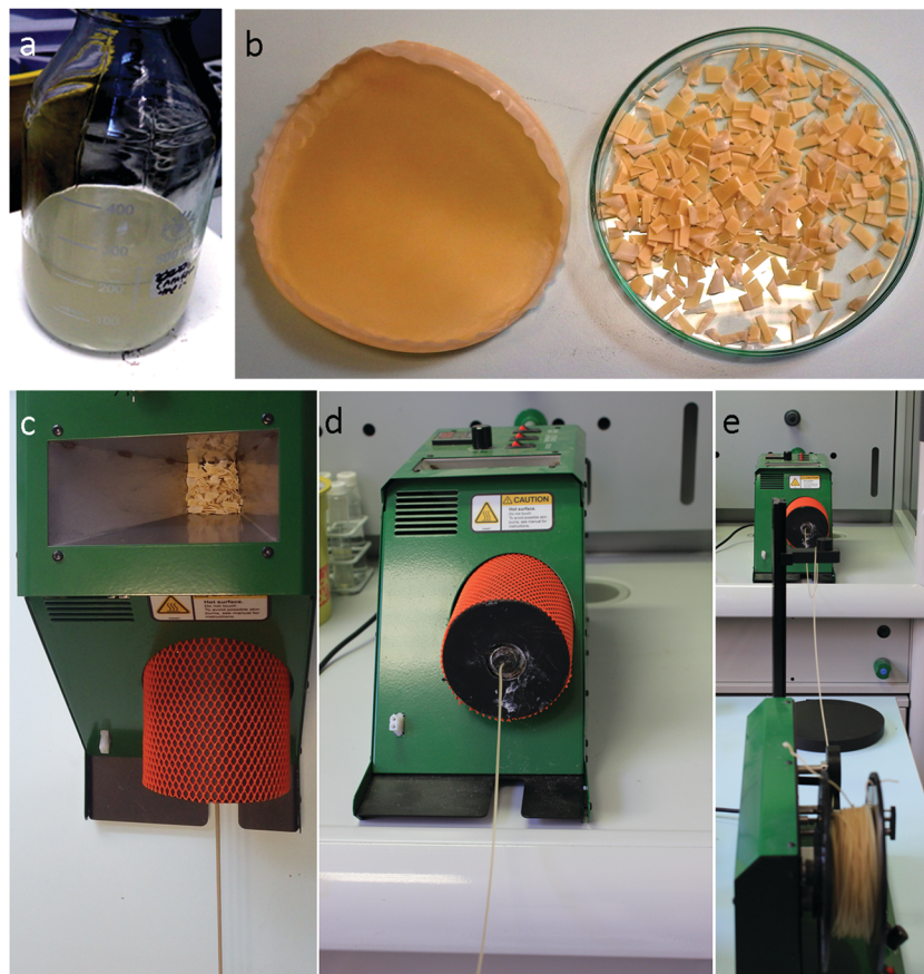
Fig. 1 (a) PCL and SA in DCM; (b) cast and cut film and (c)–(e) extrusion method to create filaments of PCL/SA.
