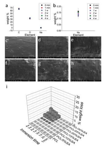
Fig. 2 PCL/15%SA filament at time intervals in water (a) and (b) EDX analysis of C, O and Na elemental weight% concentration; SEM images (500  $\mu$ m scale bar) (c)–(h) 0 min, 1 min, 1 w, 2 w, 3 w and 4 w, respectively; and (i) % weight loss versus time of PCL/5-30%SA in deionised water.
