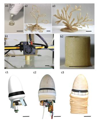
Fig. 6 (a1) 3D pen with PCL/15%SA; (a2) and (a3) 3D pen plant-like and macroalgae-like structures with PCL/15%SA; (b1) and (b2) 3D printed PCL/ 15%SA; (c1) CAD model of the growing robot; and (c2) and (c3) PCL/15%SA deposition in the growing robot. Scale bars = 2 cm.
