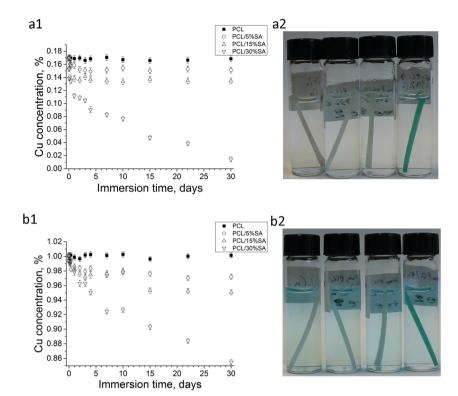
Fig. 5 % concentration of Cu vs. immersion time of the PCL/5–30%SA filament in 6 mL of (a1) 0.17% and (b1) 1% w/w Cu<sub>2</sub>SO<sub>4</sub> solution. Photographs of the PCL, PCL/5%SA, PCL/15%SA and PCL/30%SA filaments (from left to right) in the (a2) 0.17% and (b2) 1% w/w Cu<sub>2</sub>SO<sub>4</sub> water solution after 30 days of immersion.
