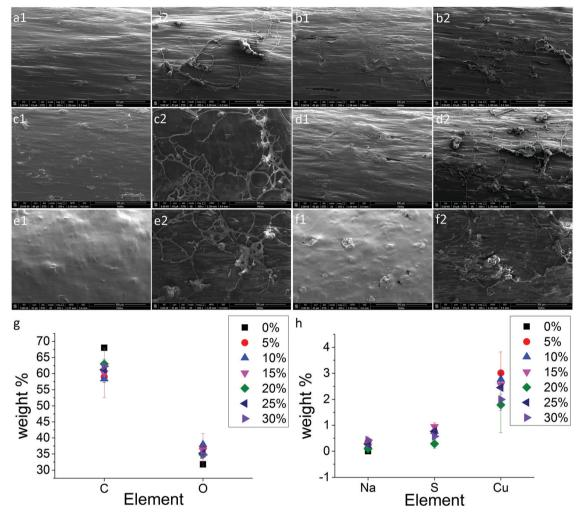
Fig. 4 SEM of (a) PCL/30%SA, (b) PCL/10%SA, (c) PCL/15%SA, (d) PCL/20%SA, (e) PCL/25%SA, and (f) PCL/30%SA where 1 denotes before Cu adsorption and 2 denotes after 4 hours of Cu adsorption; and (g) and (h) EDX elemental analysis of PCL and PCL/5-30%SA filaments.
