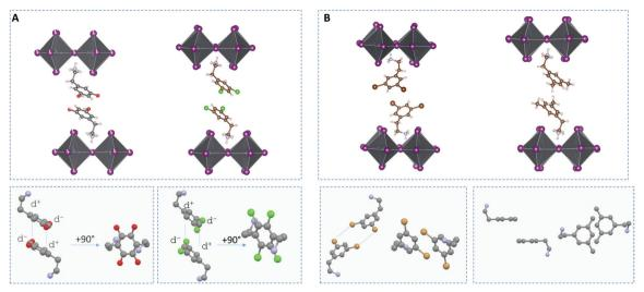
Fig. 3 Top: Partial crystal structure showing only two or three cations per four octahedra. Bottom: Cations showing the close approaches attributed to (A) dipole-dipole interaction (dY-PEA)<sub>2</sub>PbI<sub>4</sub>, where Y = F, Cl and (B) Br···Br and CH<sub>3</sub>···CH<sub>3</sub> van der Waals interactions in (dBr-PEA)<sub>2</sub>PbI<sub>4</sub> (Br-Br distance 4.15 Å) and (dMe-PEA)<sub>2</sub>PbI<sub>4</sub> (C-C distance 3.94 Å).
