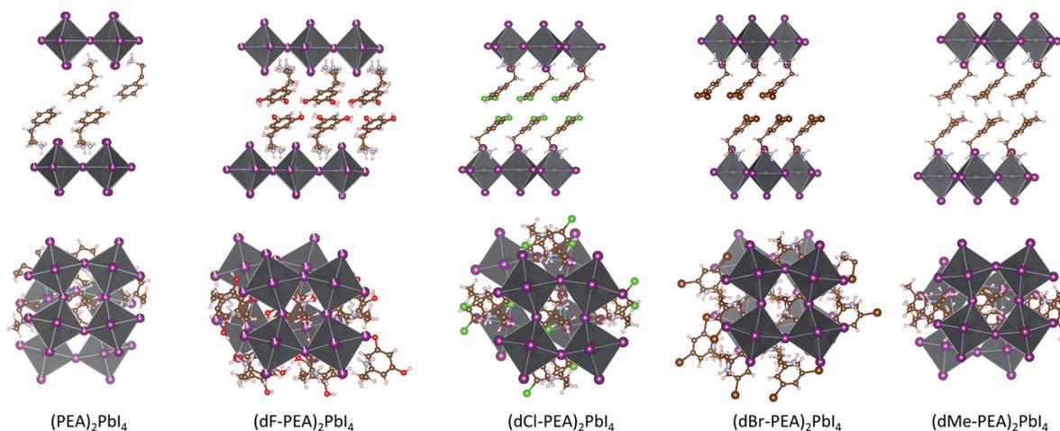
**Fig. 2** Crystal structure of  $(\text{dY-PEA})_2\text{PbI}_4$ ,  $\text{Y} = \text{H, F, Cl, Br, Me}$ , viewed along the plane of the inorganic sheet and after  $+90^\circ$  rotation around the long in-layer axis. The structure of  $(\text{PEA})_2\text{PbI}_4$  is taken from the literature.<sup>34</sup>
