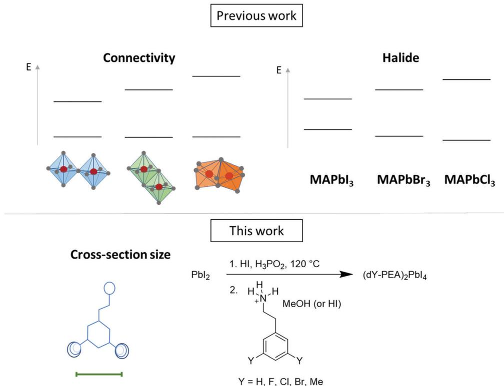
**Fig. 1** Top: Approaches to tuning the band energies of HOIPs. Trends in both excitonic and interband transitions of 2D and 3D HOIPs correlate well with the energy separation between valence and conduction bands within a series. Bottom: Approach presented here, where the width (atom–atom distance) of the cation is varied.
