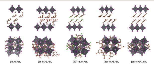
Fig. 2 Crystal structure of (dY-PEA)<sub>2</sub>PbI<sub>4</sub>, Y = H, F, Cl, Br, Me, viewed along the plane of the inorganic sheet and after +90° rotation around the long in-layer axis. The structure of (PEA)<sub>2</sub>PbI<sub>4</sub> is taken from the literature.<sup>34</sup>
