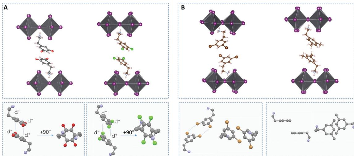
**Fig. 3** Top: Partial crystal structure showing only two or three cations per four octahedra. Bottom: Cations showing the close approaches attributed to (A) dipole–dipole interaction ( $dY$ -PEA) $_2$ PbI $_4$ , where  $Y = F, Cl$  and (B)  $Br \cdots Br$  and  $CH_3 \cdots CH_3$  van der Waals interactions in ( $dBr$ -PEA) $_2$ PbI $_4$  ( $Br$ – $Br$  distance 4.15 Å) and ( $dMe$ -PEA) $_2$ PbI $_4$  ( $C$ – $C$  distance 3.94 Å).
