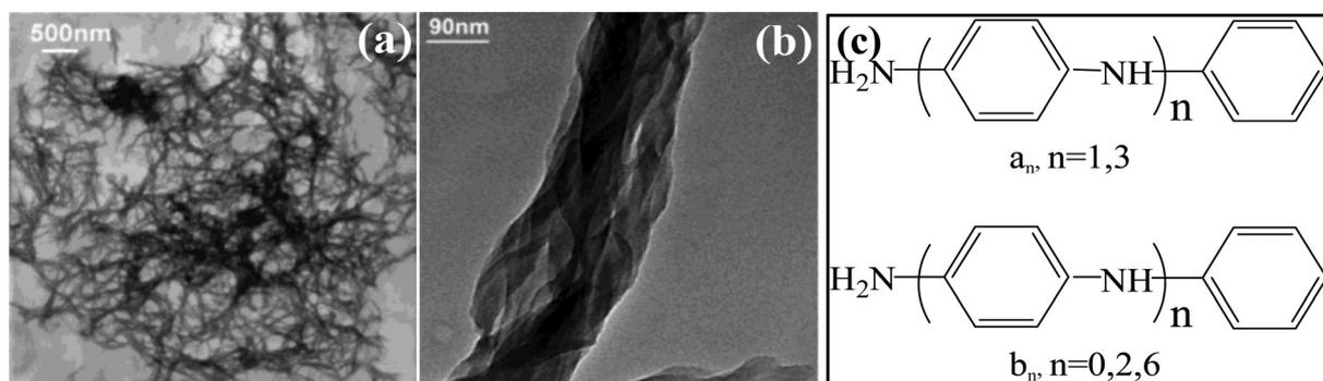
**Fig. 2** (a and b) TEM micrograph of the chiral PANI nanofiber network (a) and magnification of a fiber bundle with embedded helical nanofibers (b). (c) Molecular structures of phenylamine-capped oligomers ( $a_n$ ) and amine-amine-capped oligomers ( $b_n$ ). Reprinted with permission from ref. 38. Copyright 2004 American Chemical Society.
