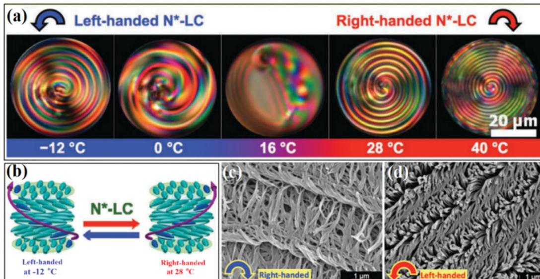
**Fig. 10** (a) Chiral inversion in the spiral optical patterns of  $N^*$ -LC during the heating and cooling processes. (b) Schematic illustration of the chiral inversion of  $N^*$ -LC. (c and d) SEM images of the H-PA films synthesized in  $N^*$ -LCs at (c)  $-12$  and (d)  $28$  °C. Reprinted with permission from ref. 60. Copyright 2020 John Wiley and Sons.
