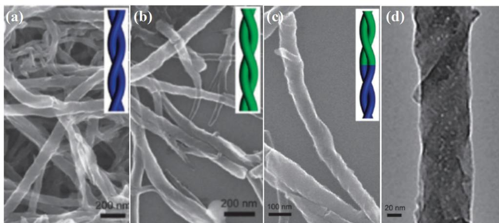
Fig. 4 (a and b) SEM images of helical PANI nanofibers obtained using (a) *R*-CSA and (b) *S*-CSA as the dopants at  $[N\text{-An}]/[\text{An}] = 1:2.5$ , respectively. (c) SEM and (d) TEM images of PANI helical heterojunctions obtained using *R*-CSA as the dopant at  $[N\text{-An}]/[\text{An}] = 1:2.5$ . Reprinted with permission from ref. 42. Copyright 2012 Royal Society of Chemistry.
