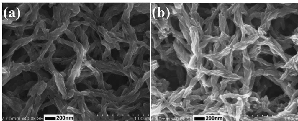
Fig. 1 (a and b) SEM images of helical PANI nanofibers prepared by the electropolymerization of aniline in the presence of *S*-CSA (a) and *R*-CSA (b) as the dopants. Reprinted with permission from ref. 29. Copyright 2010 Elsevier.
