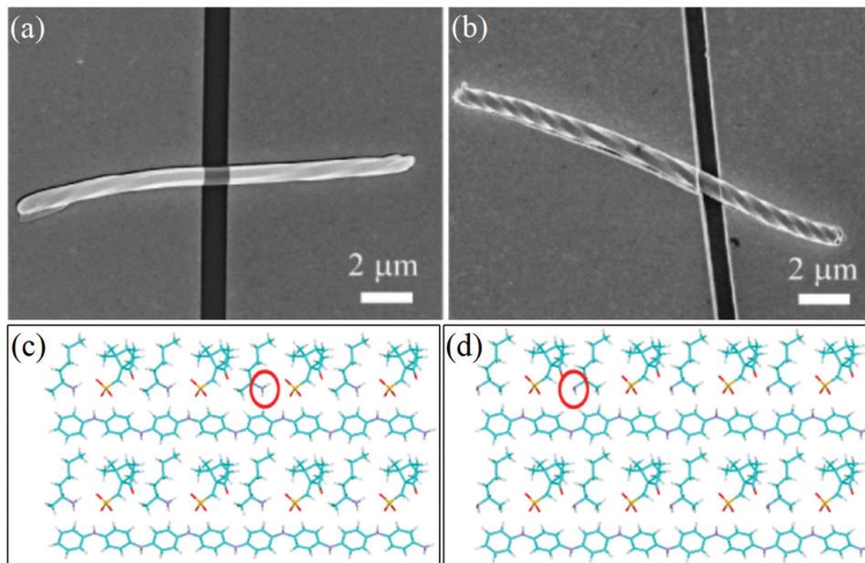
**Fig. 14** (a and b) SEM image of left-handed (a) and right-handed (b) single-helical microfiber-based enantioselective sensors. (c and d) Theoretical analysis of the enantioselective discrimination ability: (c) PANI-S-CSA inserted by *S*-2-aminohexane; (d) PANI-S-CSA inserted by *R*-2-aminohexane. Reprinted with permission from ref. 47. Copyright 2014 American Chemical Society.
