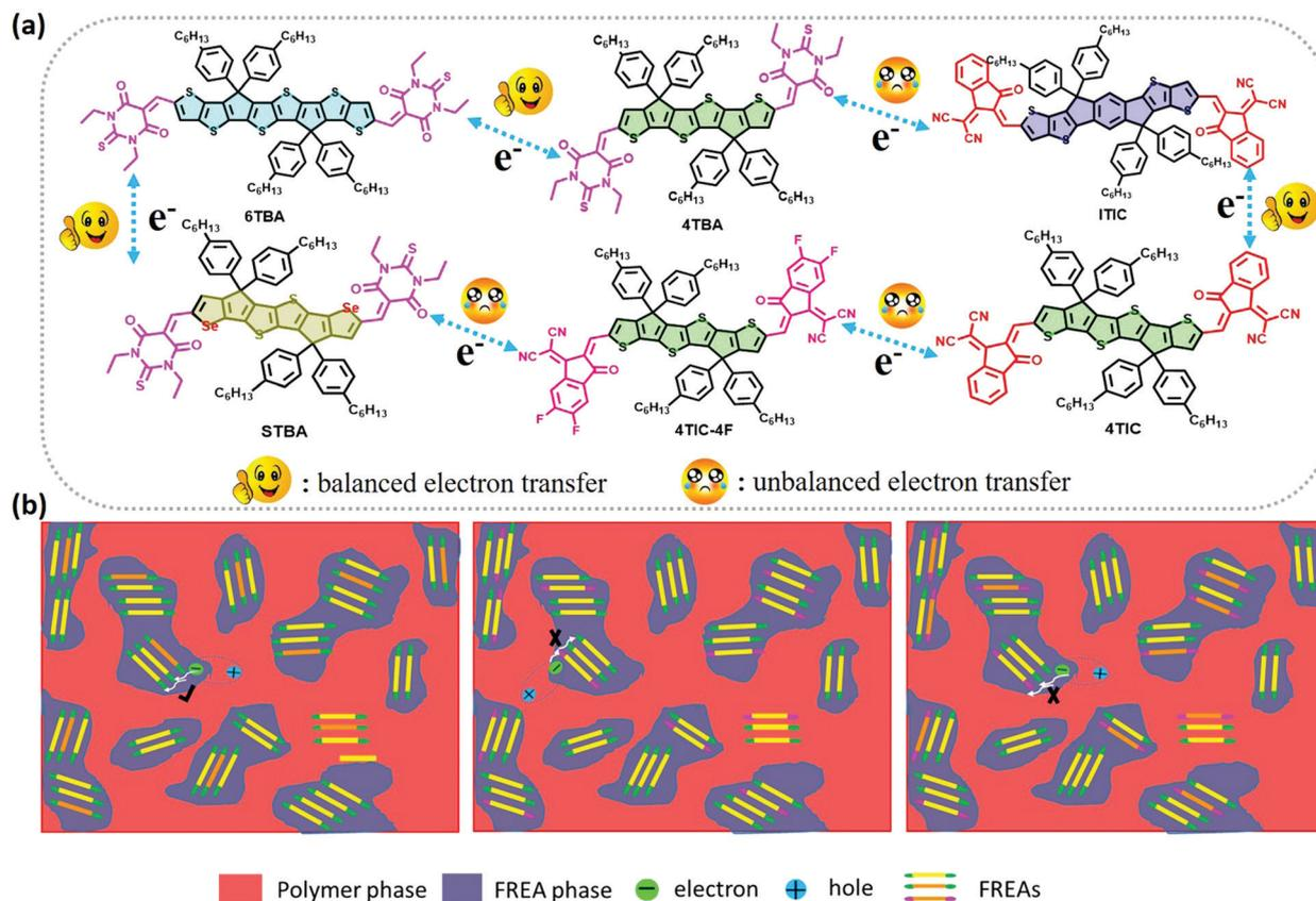
Fig. 6 (a) Hypothetical mechanism diagram of electron transport in ternary blends reflected by molecular structures. (b) The possible charge transport pathway existing in three different types of ternary systems; the yellow and orange segments in FREAs represent the donor cores, the green and pink segments represent terminals and different colors represent different donor cores or terminals.
