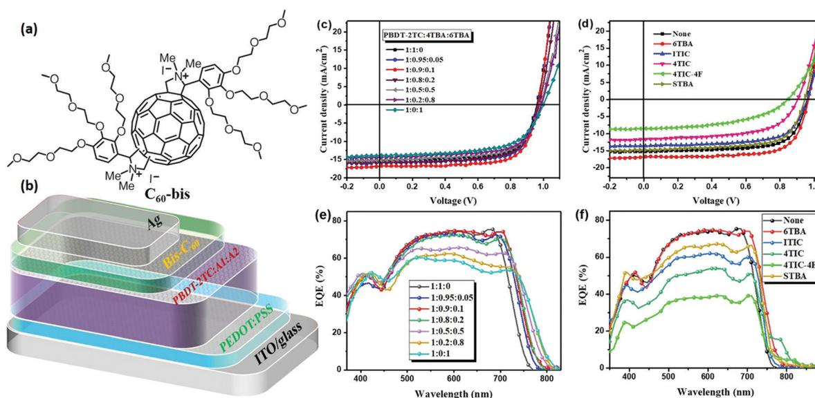
**Fig. 3** (a) Molecular structure of C<sub>60</sub>-bis. (b) Device architecture. (c)  $J$ - $V$  curves of PBDB-2TC:4TBA:6TBA based OSCs with different acceptor contents. (d)  $J$ - $V$  curves of multiple ternary system based OSCs (PBDB-2TC:4TBA:acceptor2 = 1:0.9:0.1). (e and f) EQE spectra of the respective ternary devices.
