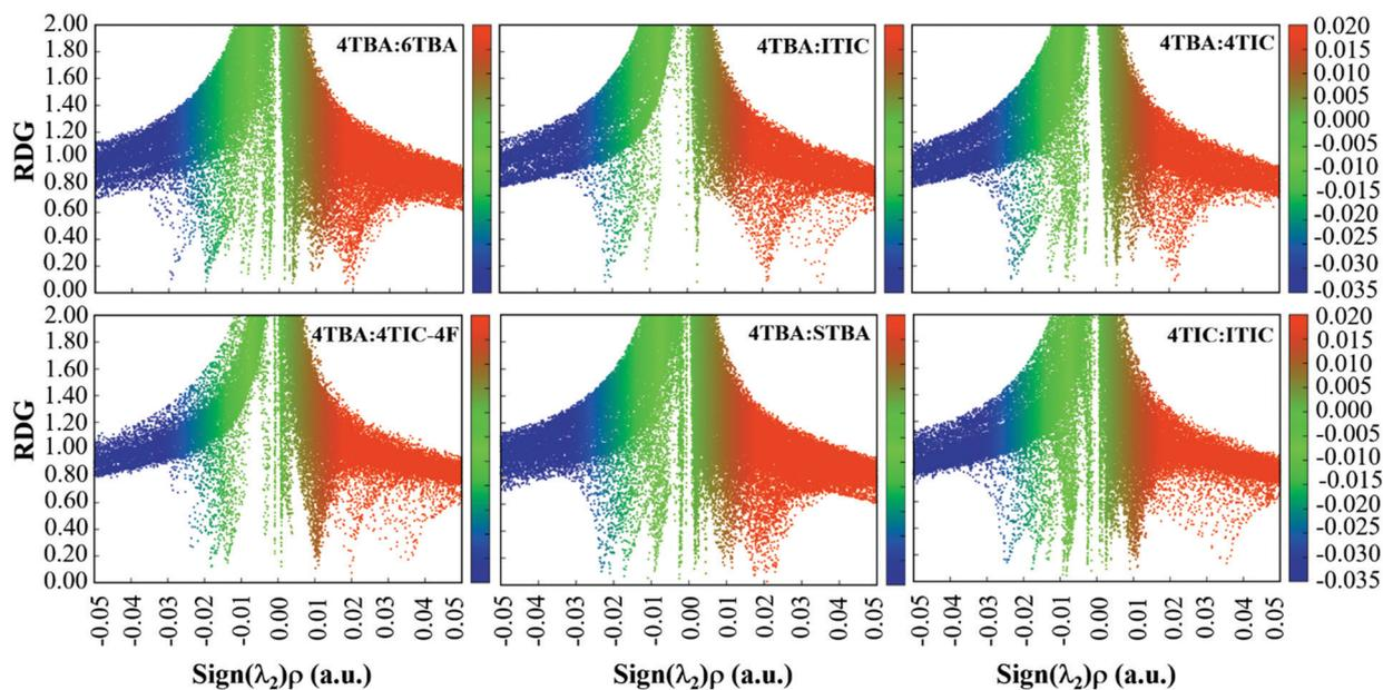
Fig. 7 The plots of the production of electron density  $\rho(r)$  and the sign of the second Hessian eigenvalue  $\lambda_2$  versus RDG for six combinations of 4TBA:6TBA, 4TBA:ITIC, 4TBA:4TIC, 4TBA:4TIC-4F, 4TBA:STBA and 4TIC:ITIC.
