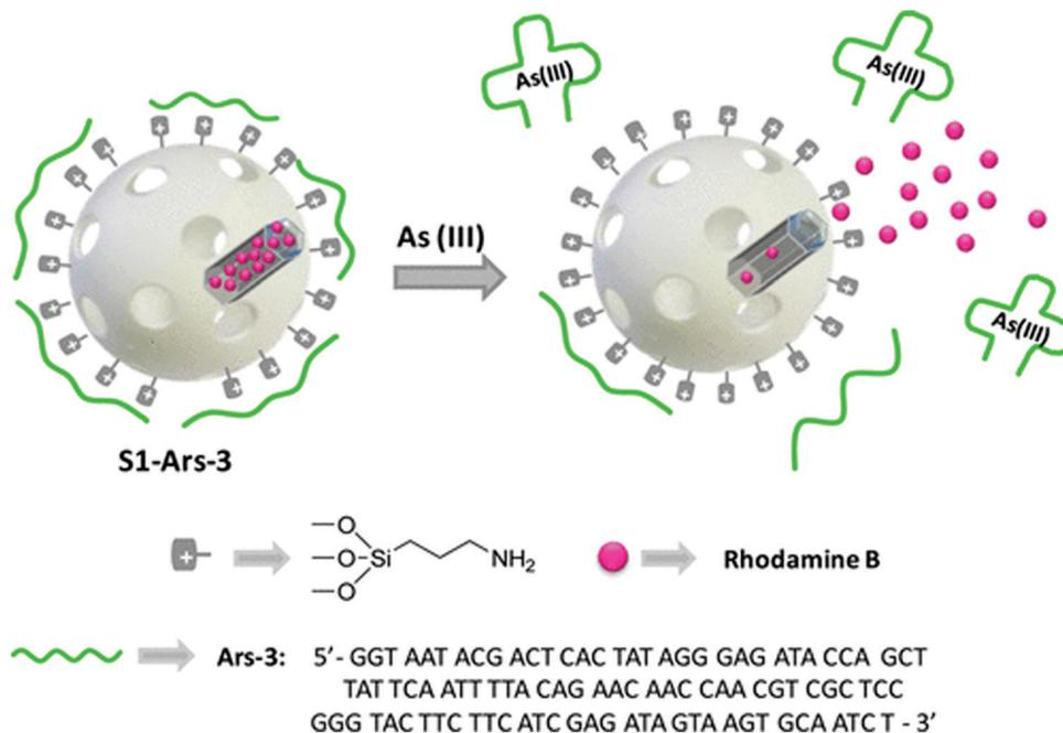
**Fig. 10** Representation of the gated material S1-Ars-3 functionalized with aminopropyl moieties and capped with Ars-3 aptamer. Delivery of the entrapped dye (rhodamine B) is specifically accomplished in the presence of As(III). Image reprinted from ref. 114 with permission. Copyright 2014 American Chemical Society.
