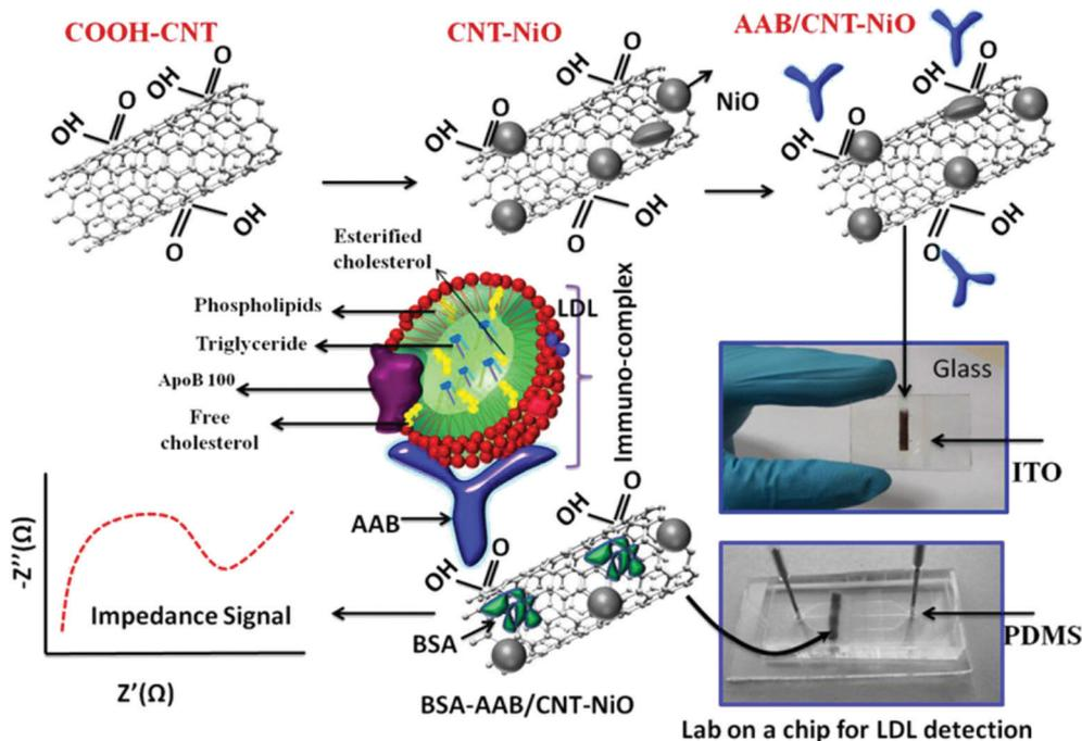
Fig. 8 Schematic representation of the lab-on-a-chip fabrication for LDL detection. Image reprinted from ref. 94 with permission. Copyright 2015 American Chemical Society.
