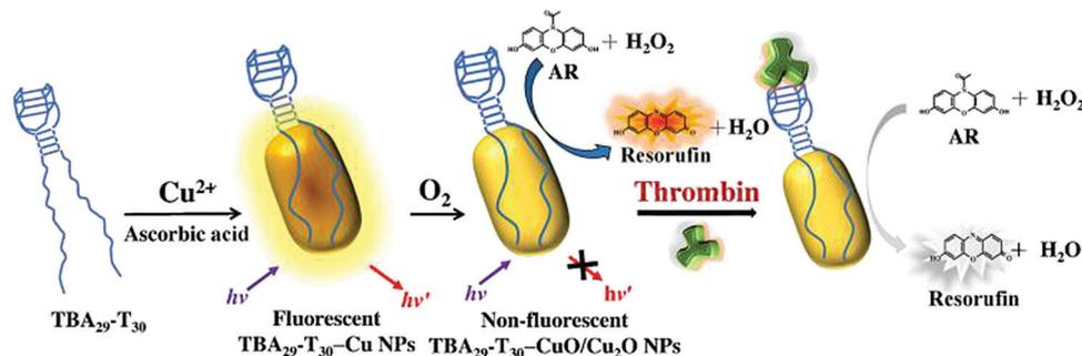
Fig. 4 Schematic representation of the preparation of Apt-CuO/Cu<sub>2</sub>O NPs exhibiting peroxidase-like catalytic activity, and their application in the determination of thrombin based on inhibition of its enzymatic activity using H<sub>2</sub>O<sub>2</sub>/AR redox system as fluorescent transducer. Image reprinted from ref. 75 with permission. Copyright 2015 Elsevier.
