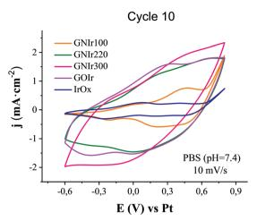
Fig. 6 Cyclic voltammetry (10th cycle) in sodium phosphate buffer, pH 7.4, of GNIr hybrid coatings in comparison with GOIr and IrOx coatings  $(10 \text{ mV s}^{-1}).$
