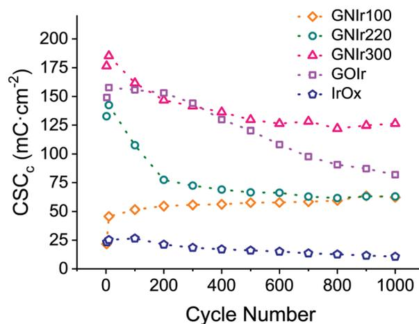
Fig. 8 Cathodic CSC evolution during cycling for IrO<sub>x</sub> (blue), GOIr (grey), GNiR100 (yellow), GNiR220 (green) and GNiR300 (red).
