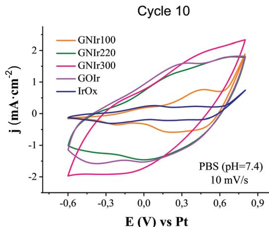
Fig. 6 Cyclic voltammetry (10th cycle) in sodium phosphate buffer, pH 7.4, of GNiR hybrid coatings in comparison with GOIr and IrO<sub>x</sub> coatings (10 mV s<sup>-1</sup>).
