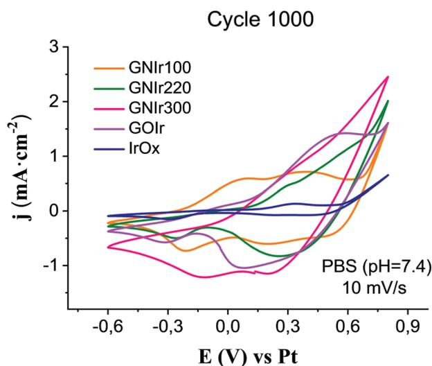
Fig. 7 Cyclic value. GNiR220 detaches from the electrode for voltammetry for each preparation of GNiR hybrids after 1000 cycles, in comparison with cycled IrO<sub>x</sub> and GOIr hybrid (10 mV s<sup>-1</sup>).
