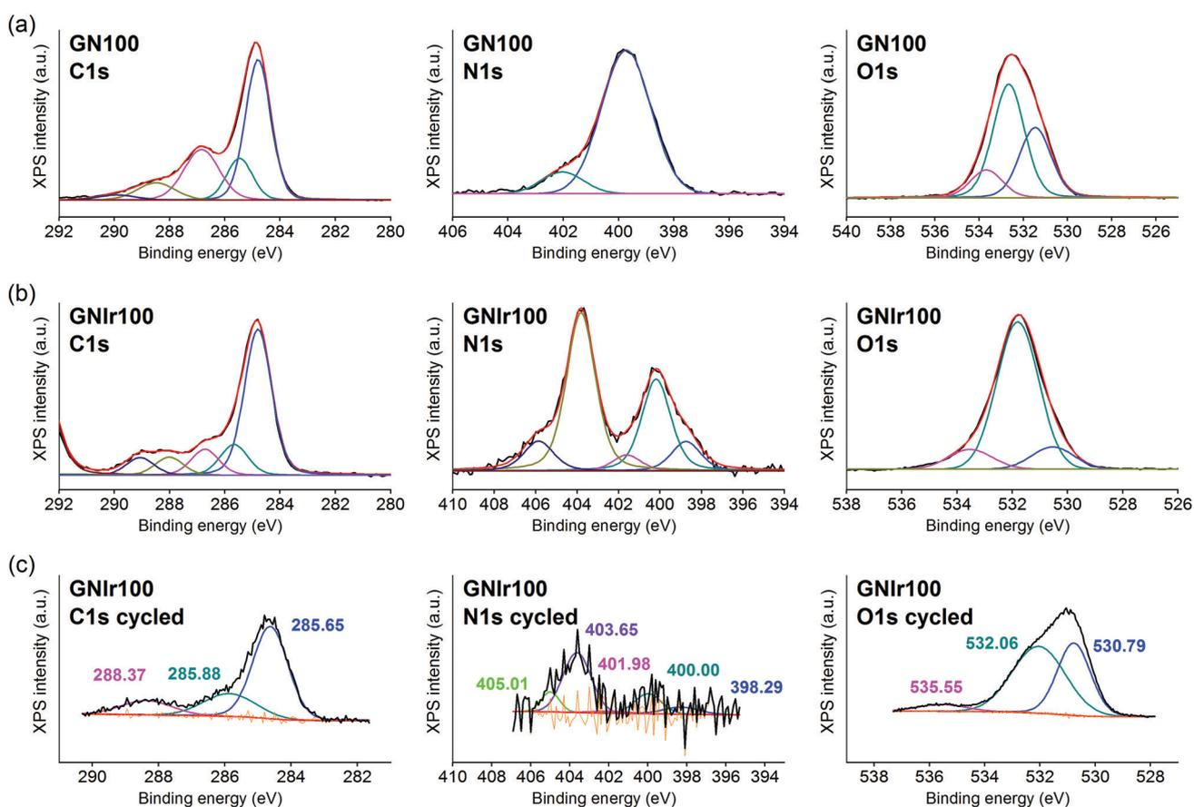
**Fig. 3** C 1s, N 1s and O 1s XPS signals for the (a) GN100 precursor and (b) the hybrid GNIr100. For ease of comparison, C 1s, N 1s and O 1s for the electrochemically cycled coating (c) is also included.
