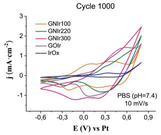
Fig. 7 Cyclic value. GNIr220 detaches from the electrode for voltammetry for each preparation of GNIr hybrids after 1000 cycles, in comparison with cycled  $IrO_x$  and GOIr hybrid (10 mV s<sup>-1</sup>).
