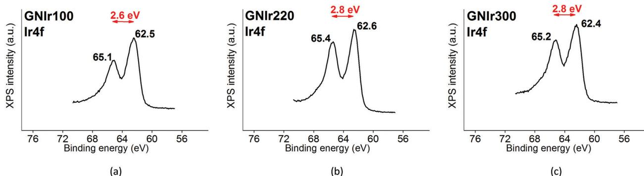
**Fig. 2** Ir 4f signal in each of the GNIr hybrids: (a) GNIr100, (b) GNIr220, (c) GNIr300.
