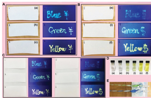
Fig. 4 Fluorescence intensity changes upon changes in temperature and solvents. (A) Application of DSA-G ⊂ H1-4C4P (a, h, c) and (B) DSA-G ⊂ H2-2C4P (e, i, f) written on filter paper, (left: under natural light, right: under ultraviolet light, \lambda_{em} = 365 nm) as tunable fluorescent inks. (C) Fluorescent inks of DSA-G ⊂ H1-4C4P (a, h, c) and DSA-G ⊂ H2-2C4P (e, i, f) on the same white paper; (a: H1-4C4P ([ H1-4C4P ] = 50 \mu M); h: DSA-G ⊂ H1-4C4P ([ H1-4C4P ] = 50 \mu M, [ DSA-G ] = 10 \mu M); c: DSA-G ⊂ H1-4C4P ([ H1-4C4P ] = 50 \mu M, [ DSA-G ] = 100 \mu M); e: H2-2C4P ([ H2-4C4P ] = 50 \mu M); i: DSA-G ⊂ H2-2C4P ([ H2-2C4P ] = 50 \mu M, [ DSA-G ] = 10 \mu M); f: DSA-G ⊂ H2-2C4P ([ H2-2C4P ] = 50 \mu M, [ DSA-G ] = 100 \mu M)). Images of (D) the solutions and (E) solution-loaded pens.
