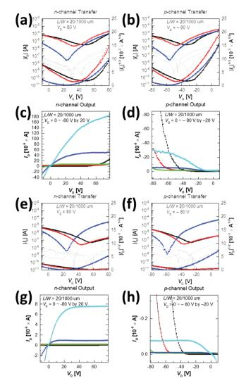
Fig. 7 (a, b, e and f) Transfer and (c, d, g and h) output characteristics of the n-type and p-type devices of (a-d) P1 and (e-h) P2 under different annealing conditions: 100 °C (black), 200 °C (red) and 300 °C (blue).
