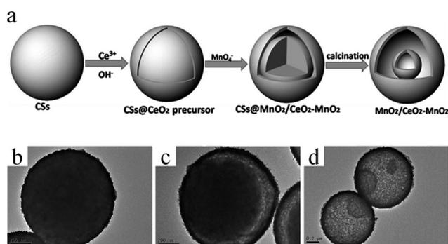
**Fig. 12** (a) Schematic illustration of the synthesis process of  $\text{MnO}_2/\text{CeO}_2\text{-MnO}_2$  double-shelled hollow spheres. TEM images of (b) CSs@ $\text{CeO}_2$  precursor core-shell spheres, (c) yolk-shell CSs@ $\text{MnO}_2/\text{CeO}_2\text{-MnO}_2$ , and (d)  $\text{MnO}_2/\text{CeO}_2\text{-MnO}_2$  double-shelled hollow spheres. Reprinted from ref. 52 with kind permission.
