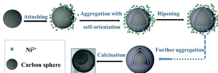
Fig. 10 Plausible formation process of multishelled NiO microspheres. Reproduced from ref. 45 with permission.
