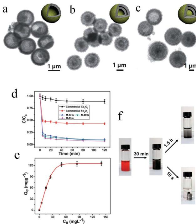
Fig. 47 TEM images of M-MHs: (a) M-SHs, (b) M-DHs, and (c) M-THs. (d) Adsorption rates of Congo red on the three M-MHs, commercial  $\gamma\text{-Fe}_2\text{O}_3$ , and commercial  $\text{Co}_3\text{O}_4$ . (e) Adsorption isothermal curves of Congo red on M-THs. (f) Photographs confirming the absorption of Congo red by M-THs with time. Reproduced from ref. 240 with kind permission.
