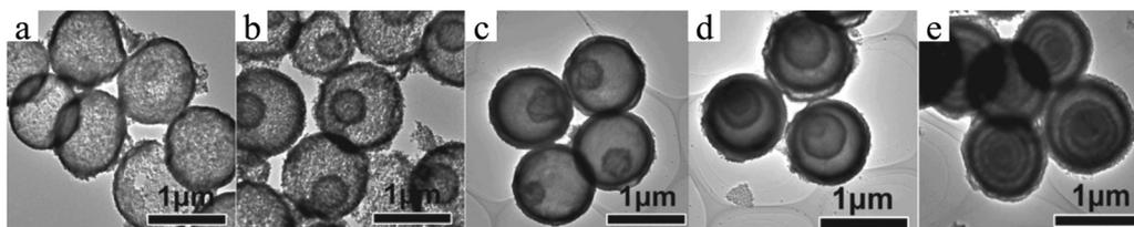
Fig. 7 TEM images of (a) single-, (b) double-, (c) triple-, (d) quadruple-, and (e) quintuple-shelled hollow SnO<sub>2</sub> microspheres prepared by a one-step thermal treatment process using alkali-treated carbonaceous microspheres as the hard template. Reprinted from ref. 38 with kind permission.
