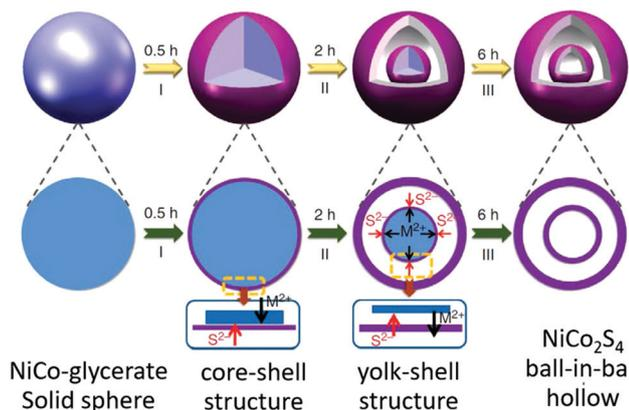
Fig. 29 Schematic illustration of the preparation of double-shelled  $\text{NiCo}_2\text{S}_4$  ball-in-ball hollow spheres via the sulfidation of NiCo glycerate solid spheres. Reprinted from ref. 39 with permission.
