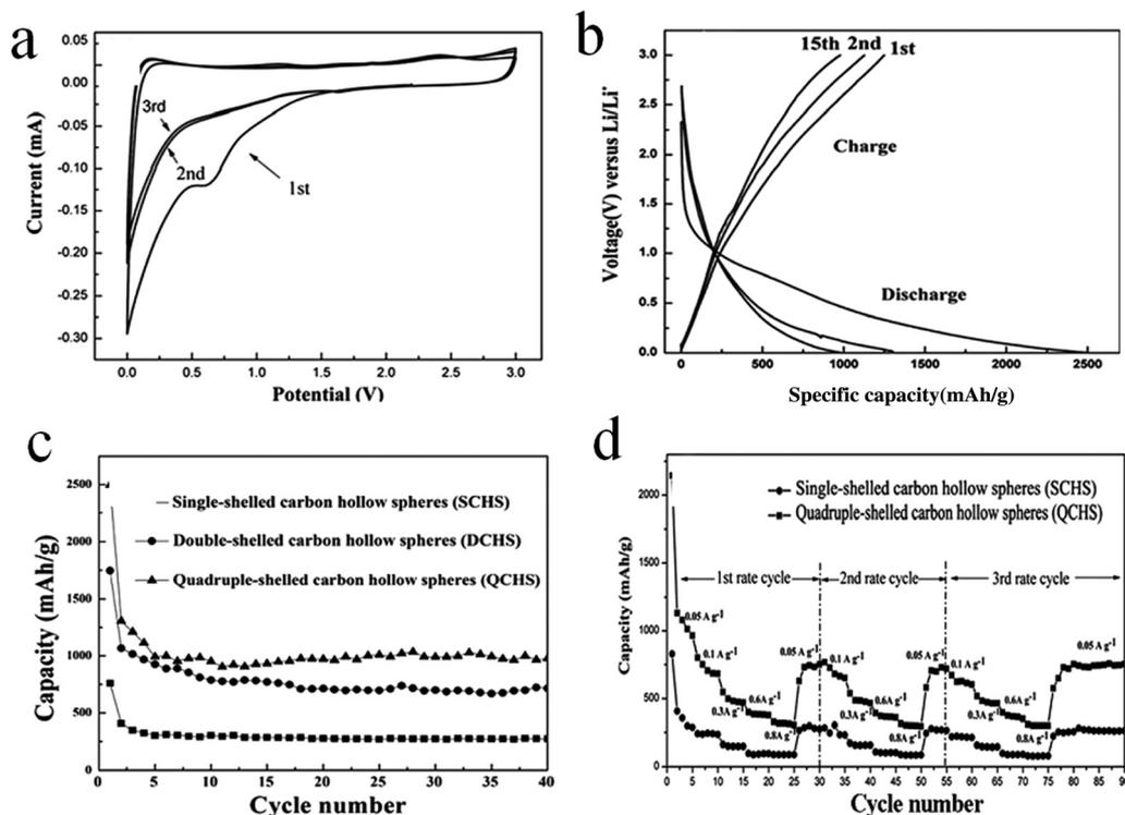
Fig. 40 (a) CV curves of the first 3 cycles and (b) GCD curves at 50 mA g<sup>-1</sup> for the quadruple-shelled carbon hollow spheres. (c) Cycling performances of carbon hollow spheres for different numbers of shells. (d) Rate capability of quadruple- and single-shelled carbon hollow spheres at various current densities. Reproduced from ref. 27 with permission.
