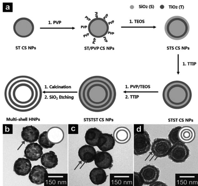
Fig. 2 (a) Schematic illustration of the synthesis of multishelled porous  $\text{TiO}_2$  hollow nanoparticles using  $\text{SiO}_2$  as the hard template. Typical TEM images of single-shelled (b), double-shelled (c), and triple-shelled (d) hollow  $\text{TiO}_2$  nanospheres. Reprinted from ref. 19 with permission. Copyright 2019 John Wiley & Sons.
