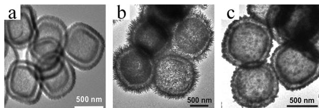
Fig. 3 Schematic illustration of the synthesis procedure of  $\text{NiS}$  box-in-box hollow structures. TEM images of the box-in-box hollow structures:  $\text{NiS}$  (a),  $\text{CuS}$  (b), and  $\text{MnS}$  (c). Reprinted from ref. 24 with kind permission.
