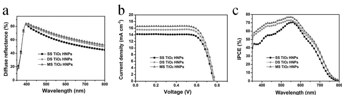
Fig. 41 (a) Diffuse reflectance spectra, (b) current density–voltage characteristics ( $J$ - $V$  curves), and (c) IPCEs of SS- $\text{TiO}_2$ -HNPs (square), DS- $\text{TiO}_2$ -HNPs (circle), and MS- $\text{TiO}_2$ -HNPs (triangle). Reprinted from ref. 22 with kind permission.
