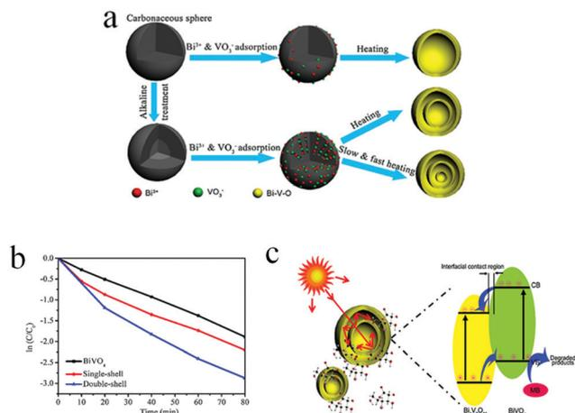
Fig. 44 (a) Schematic illustration of the synthesis procedure of multi-shelled Bi-V-O hollow microspheres. (b) Catalytic performance of solid BiVO<sub>4</sub> and single- and double-shelled Bi-V-O hollow microspheres. (c) Schematic diagram of the photocatalytic mechanism of the heterostructures of multishelled Bi-V-O hollow microspheres. Reprinted from ref. 234 with kind permission.
