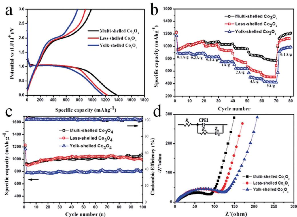
Fig. 36 Electrochemical performance of  $\text{Co}_3\text{O}_4$  hollow spheres in yolk-shell, fewer-shelled, and multishelled structures when used as the anode for LIBs. (a) Initial charge-discharge curves, (b) rate capability for different current densities, (c) cycling performance at  $1 \text{ A g}^{-1}$ , and (d) electrochemical impedance spectra. Reproduced from ref. 169 with permission.
