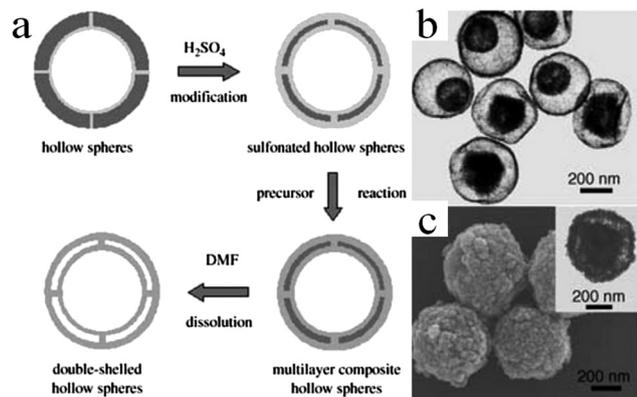
Fig. 13 (a) Schematic illustration of the synthesis of double-shelled inorganic hollow spheres. (b) TEM images of double-shelled  $\text{TiO}_2$  hollow spheres and (c) SEM and TEM images (inset) of  $\text{Fe}_3\text{O}_4$ . Reprinted from ref. 53 with kind permission.
