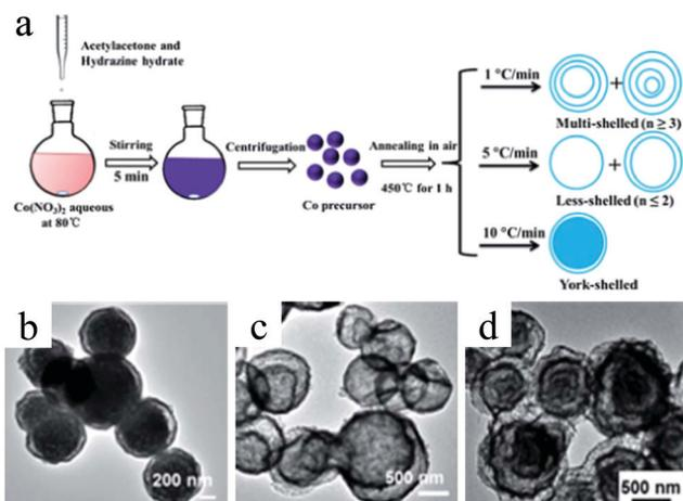
Fig. 35 (a) Schematic illustration of the synthesis process and (b–d) typical TEM images of  $\text{Co}_3\text{O}_4$  hollow spheres in yolk-shell, fewer-shelled, and multishelled structures. Reproduced from ref. 169 with permission.
