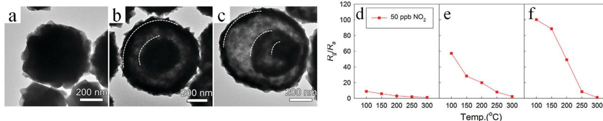
Fig. 43 TEM images of (a) D-WO<sub>3</sub>, (b) 2S-WO<sub>3</sub>, and (c) 3S-WO<sub>3</sub>. Gas responses ( $R_g/R_a$ ) to 50 ppb NO<sub>2</sub> of (d) D-WO<sub>3</sub> spheres, (e) 2S-WO<sub>3</sub> spheres, and (f) 3S-WO<sub>3</sub> spheres. Reprinted from ref. 223 with kind permission.
