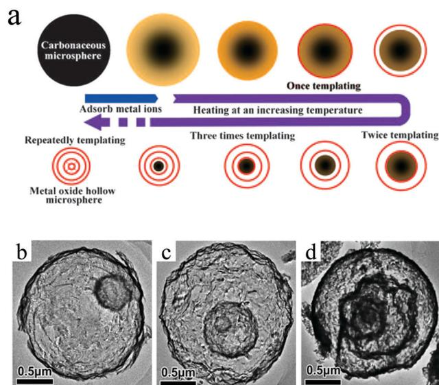
Fig. 5 (a) Schematic diagram of the sequential template strategy to multishelled metal oxide hollow microspheres. TEM images of double-shelled (b), triple-shelled (c), and quadruple-shelled (d)  $\alpha$ -Fe<sub>2</sub>O<sub>3</sub> hollow microspheres. Reprinted from ref. 28 with kind permission.
