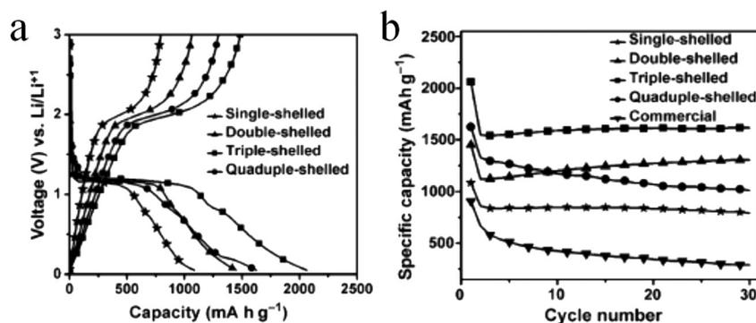
Fig. 34 (a) Initial discharge–charge curves for  $\text{Co}_3\text{O}_4$  hollow microspheres with different numbers of shells. (b) Discharge capacity versus number of cycles for  $\text{Co}_3\text{O}_4$  hollow microspheres with different numbers of shells and commercial  $\text{Co}_3\text{O}_4$ . Reprinted from ref. 40 with permission. Copyright 2013 John Wiley & Sons.
