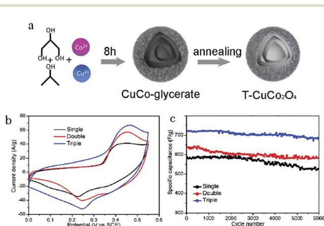
Fig. 39 (a) Schematic illustration of the preparation of  $\text{T-CuCo}_2\text{O}_4$ . (b) CV curves at  $50 \text{ mV s}^{-1}$  and (c) cycling performance of  $\text{CuCo}_2\text{O}_4$  hollow microspheres with different numbers of shells as an anode for LIBs. Reproduced from ref. 183 with permission.
