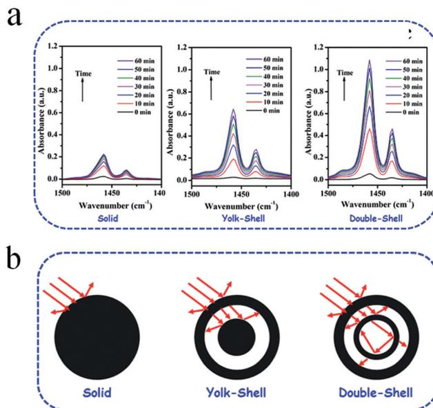
Fig. 45 Comparison of the diffusion characteristics of *o*-DCB (a) and light diffusion (b) over solid, yolk-shell, and double-shelled ZnFe<sub>2</sub>O<sub>4</sub> spheres. Reprinted from ref. 236 with permission.
