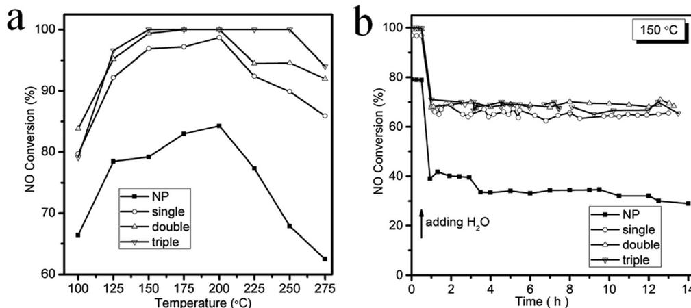
Fig. 46 NO conversion of the  $\text{CeO}_2\text{-MnO}_x$  catalysts as a function of temperature in the absence of water (a) and in the presence of water at 150 °C (b). Reproduced from ref. 237 with kind permission.
