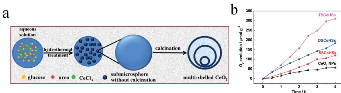
Fig. 42 (a) Proposed formation process of multishelled CeO<sub>2</sub> hollow microspheres. (b) Comparison of photocatalytic oxygen evolution performance of CeO<sub>2</sub> NPs and as-prepared multishelled CeO<sub>2</sub> hollow microspheres with different numbers of shells. Reproduced from ref. 219 with kind permission.
