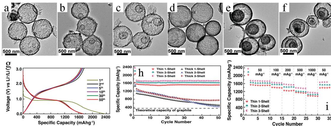
Fig. 33 (a–f) TEM images of multishelled  $\alpha$ - $\text{Fe}_2\text{O}_3$  hollow nanospheres with different numbers of shells and shell thicknesses: (a) thin single-shelled, (b) thin double-shelled, (c) thin triple-shelled, (d) thick single-shelled, (e) thick double-shelled, and (f) thick triple-shelled samples. (g–i) Electrochemical performance of above samples. Reprinted from ref. 36 with kind permission.
