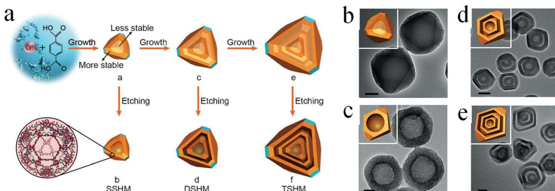
**Fig. 26** (a) Schematic illustration of the preparation procedure of multishelled hollow MIL-101 by step-by-step and post-etching processes. TEM images of solid MIL-101 (b), SSHM (c), DSHM (d), and TSHM (e). Scale bars: (b and c) 50 nm; (d and f) 200 nm. Insets in (b–e) show the corresponding FFT patterns. Reprinted from ref. 94 with kind permission.
