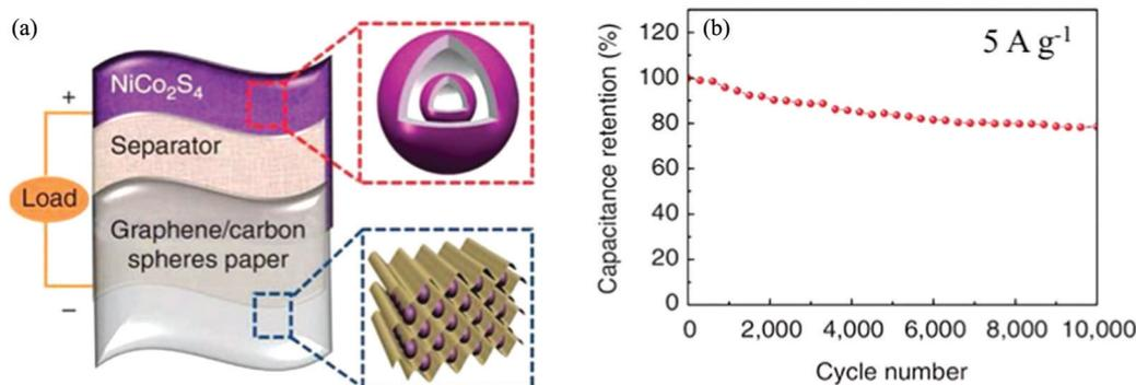
Fig. 32 (a) Schematic illustration of the ASC device based on  $\text{NiCo}_2\text{S}_4$  and graphene/carbon sphere paper. (b) Cycling performance of the ASC device at  $5 \text{ A g}^{-1}$ . Reproduced from ref. 19 with permission.
