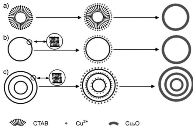
Fig. 19 Schematic of the formation mechanism of single-shelled and multishelled Cu<sub>2</sub>O hollow spheres using CTAB-assembled vesicles as the soft template. Reprinted from ref. 75 with kind permission.
