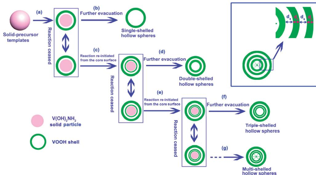
Fig. 31 Schematic illustration of the formation of VOOH hollow nanospheres with controlled numbers of shells *via* the direct thermal treatment of solid  $V(OH)_2NH_2$  nanospheres. Reprinted from ref. 110 with kind permission.
