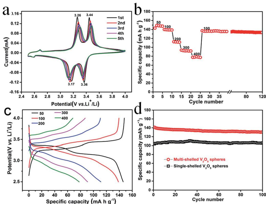
Fig. 38 Electrochemical performance of multishelled  $\text{V}_2\text{O}_5$  hollow microspheres as the anode for LIBs. (a) CV profiles at  $0.05 \text{ mV s}^{-1}$ , (b) rate performance, (c) charge–discharge curves at different current densities, and (d) cycling stability when compared with traditional single-shelled hollow samples at a current density of  $100 \text{ mA g}^{-1}$ . Reproduced from ref. 175 with permission.
