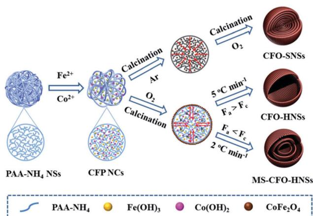
Fig. 16 Schematic illustrations of the formation processes of CFO-SNSs, CFO-HNSs, and MS-CFO-HNSs using PAA-NH<sub>4</sub> as the hard template. Reproduced from ref. 63 with permission.
