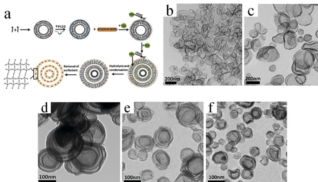
Fig. 25 (a) Formation mechanism of multishelled hollow PMO nanospheres using P123, CTAB, and SDS as a dual template with the assistance of compressed CO<sub>2</sub>. (b–f) TEM images of multishelled PMO hollow nanospheres obtained at CO<sub>2</sub> pressures of 3.90 (b), 4.40 (c), 4.90 (d), 5.60 (e), and 5.90 (f) MPa. Reproduced from ref. 88 with kind permission.
