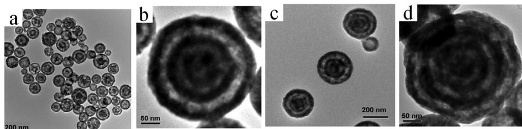
Fig. 20 TEM images of (a) double-shelled, (b and c) triple-shelled, and (d) quadruple-shelled Cu<sub>2</sub>O hollow spheres for different CTAB concentrations: (a and b) 0.13 and (c and d) 0.15 M. Reprinted from ref. 75 with kind permission.
