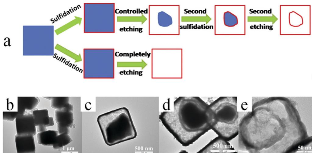
Fig. 30 (a) Schematic illustration of the synthesis procedure for the formation of double-shelled CuS hollow nanocages via the  $\text{Cu}_2\text{O}$  self-template approach. TEM images of  $\text{Cu}_2\text{O}@\text{CuS}$ : (b) before and (c) after the initial partial etching treatment. TEM images of (d)  $\text{Cu}_2\text{O}@\text{CuS}@\text{CuS}$  and (e) double-shelled CuS hollow nanocages. Reprinted from ref. 109 with kind permission.
