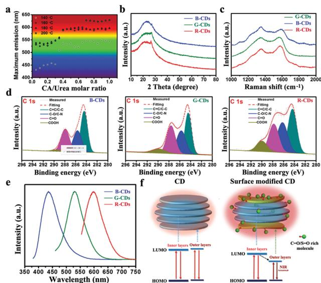
**Fig. 2** (a) Maximum emission peaks of CDs at various CA/urea molar ratios and reaction temperatures. XRD patterns (b), Raman spectra (c), high-resolution C1s XPS spectra (d), emission spectra (e) of B-CDs, G-CDs, and R-CDs. Reproduced with permission from ref. 55. Copyright 2018, Wiley-VCH. (f) Schematic of the structure and energy level of CDs and S=O/C=O-rich molecule modified CDs. Reproduced with permission from ref. 56. Copyright 2018, Wiley-VCH.
