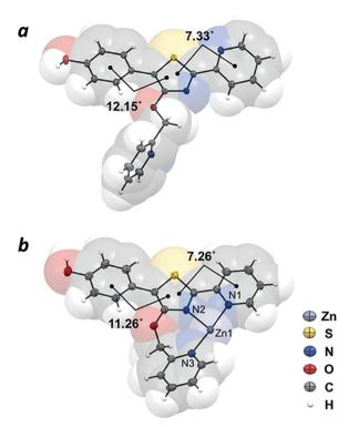
Fig. 3 X-ray crystal structures of (a) 4'-O-Pic-HPPT (4) and (b) 4-Zn(II). Nitrate counterions are omitted for clarity. Thermal ellipsoids are shown at 50% probability.
