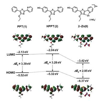
Fig. 2 DFT calculations of energy bands and spatial distributions of molecular orbital coefficients (HOMO and LUMO) for 4'-O-Et-PPT (1), 4'-O-Et-HPPT (2), and 2-Zn(II). See ESI† for additional DFT calculations.
