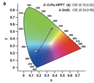
Fig. 6 (a) Spectral changes in the photoluminescence of  $\bf 4$  (30  $\mu M$  in CH<sub>3</sub>CN) upon titration of Zn(NO<sub>3</sub>)<sub>2</sub>·6H<sub>2</sub>O (3 mM in CH<sub>3</sub>CN) and excitation at the isosbestic point ( $\lambda_{\rm ex}$  = 393 nm). (b) CIE chromaticity diagram of **4** showing the progression in emitted light with Zn(NO<sub>3</sub>)<sub>2</sub> addition.
