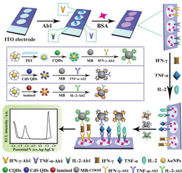
Fig. 5 Preparation and schematic illustration of the multiplexed ECL immunosensor for simultaneous detection of IFN- $\gamma$ , TNF- $\alpha$  and IL-2. Reprinted with permission from ref. 172. Copyright 2017 American Chemical Society.
