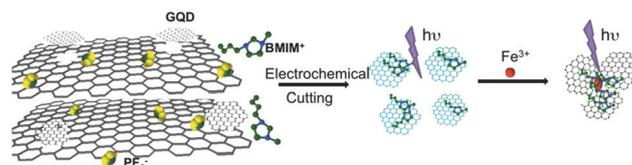
Fig. 2 Schematic illustration of GD synthesis from 3D graphene and the mechanism of Fe<sup>3+</sup> detection. Reprinted with permission from ref. 42. Copyright (2014) Wiley-VCH Verlag GmbH & Co. KGaA, Weinheim.
