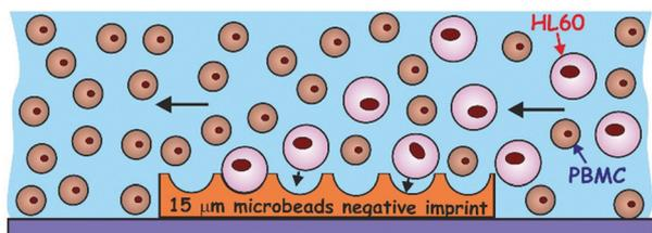
**Fig. 1** The principle of particle imprint-based AML cell depletion from a mixture with PBMCs. The substantially larger (AML) cells are preferentially attracted and retained on the imprint due to the large contact area whereas smaller, healthy PBMCs are flushed through with little interaction.
