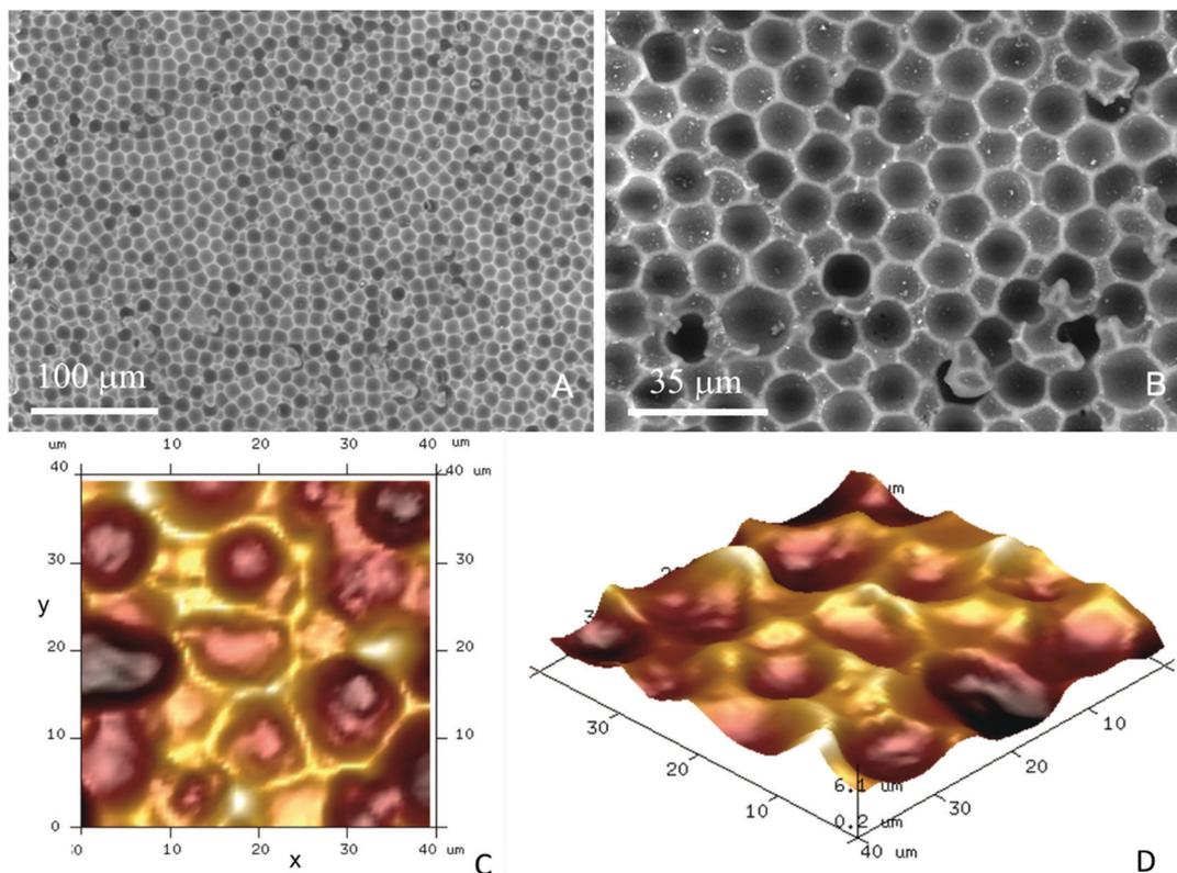
**Fig. 3** SEM images of typical negative PDMS imprints of a layer of 15  $\mu\text{m}$  PMMA microbeads (Spheromers<sup>®</sup> CA15) deposited on glass slides as a suspension. The scale bars represent (A) 100  $\mu\text{m}$  and (B) 35  $\mu\text{m}$ , respectively. (C and D) Atomic force microscope images of the CA15 particle imprints with different perspectives.
