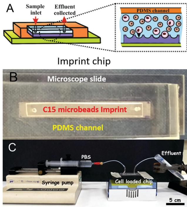
**Fig. 4** (A) Schematic and (B) top side view of the actual particle imprint (of length 4 cm and width 6 mm) attached on a microscope slide with PDMS channelled casing with input and output channels. (C) Photographs showing the setup used for the static experiment using the syringe pump, the cell loaded chip and the collected effluent.
