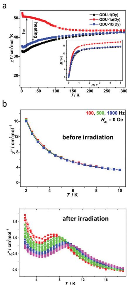
**Fig. 3** (a) Temperature dependence of  $\chi_m T$  values for QDU-1(Dy), QDU-1a(Dy) and QDU-1b(Dy); (b) plots of  $\chi'(T)$  in the absence of a dc field at various ac frequencies for QDU-1(Dy) (up) and QDU-1a(Dy) (bottom). Reproduced with permission from ref. 43. Copyright 2020 American Chemical Society.<sup>43</sup>
