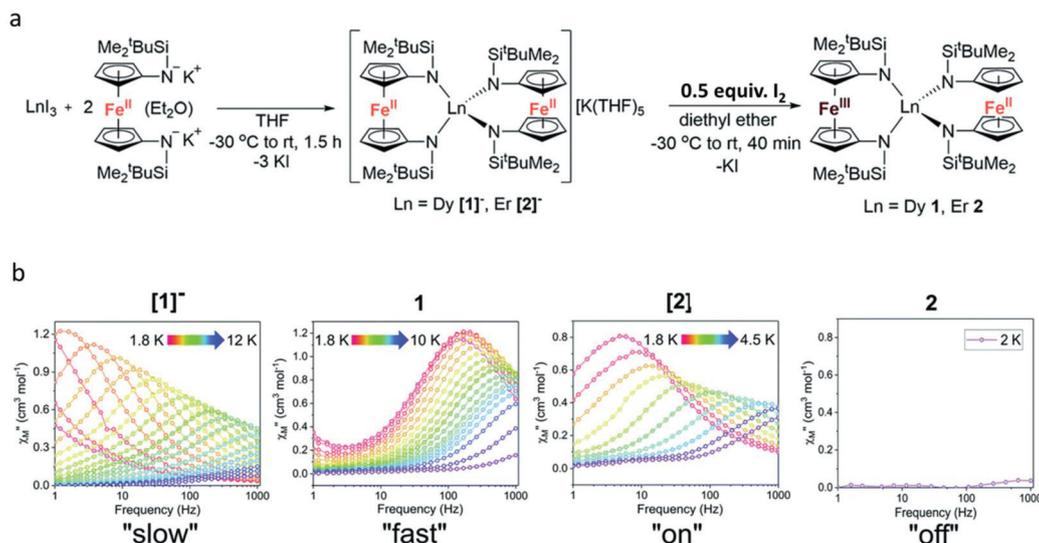
**Fig. 8** (a) Synthesis of  $[1]^-$ , **1**,  $[2]^-$ , and **2**; (b) plots of  $\chi''(\nu)$  for  $[1]^-$  and **1** under a 1000 Oe dc field and  $[2]^-$  and **2** under a 500 Oe dc field. Reproduced with permission from ref. 76. Copyright 2017 Royal Society of Chemistry.<sup>76</sup>
