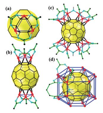
Fig. 1 The simplified structures of the synthesized cuprofullerenes. (a)  $Cu_3$  unit, (b)  $C_{60}$ @ $Cu_6$ , (c)  $C_{60}$ @ $Cu_{12}$  and (d)  $C_{60}$ @ $Cu_{24}$ . Color code: red, Cu; cyan, O; black, C; green, F; gray, H.
