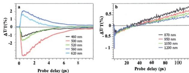
Fig. 14 Dynamics of  $\Delta T/T$  at selected probe wavelengths, at the two different time scales of energy flow in the Au clustered structures (a and b). From these data, a water dispersed Au “clustered” structure can be operated as very efficient nanoheaters whereas it was not observed in dried Au supracrystals.
