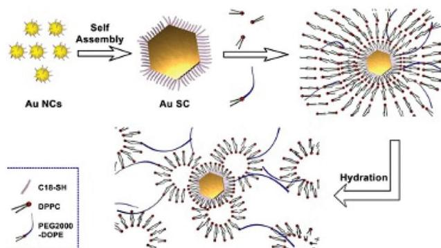
Fig. 6 Cartoon showing the procedure used to grow shaped supracrystals of a hydrophobic coating agent treated with organic molecules such as DPPC and PEG-2000-DOPE. This permits the dispersion of shaped hydrophobic supracrystals in aqueous solution.
