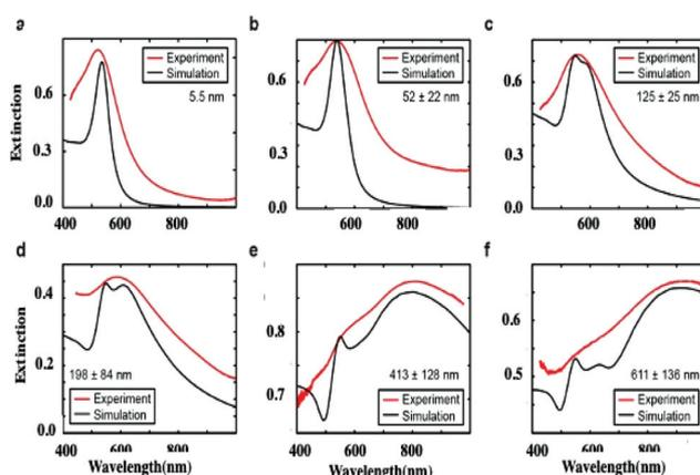
**Fig. 10** Extinction spectra of isolated Au nanocrystals and assemblies of various sizes. (a)  $5.5 \pm 0.4$  nm Au nanocrystals; Au aggregates with sizes of (b)  $52 \pm 22$  nm, (c)  $125 \pm 25$  nm, and (d)  $198 \pm 84$  nm; Au supracrystals with sizes of (e)  $413 \pm 128$  nm and (f)  $611 \pm 136$  nm. The average sizes were used to fit the measured data.
