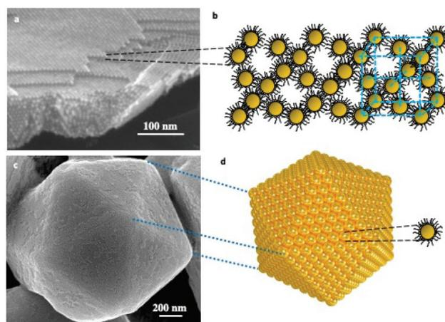
**Fig. 1** Supracrystals grown under heterogeneous (a and b) and homogeneous (c and d) conditions. SEM images of nanocrystals self-assembled layer by layer (a) and shaped supracrystals (b) of 5 nm Au nanocrystals coated with dodecanthiol. Scheme of such fcc supracrystals (b and d).
