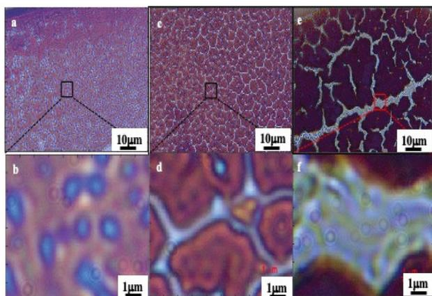
**Fig. 4** Optical micrographs of the 0.2–0.6  $\mu\text{m}$  supracrystal film, in the transmission mode. (a and b), 0.4–1.0  $\mu\text{m}$  (c and d) and 1.0–1.4  $\mu\text{m}$  (e and f).
