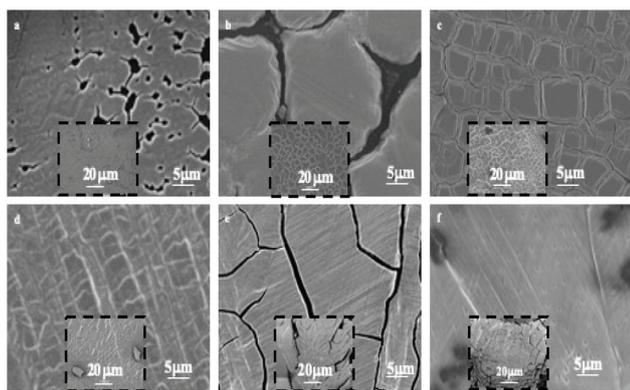
**Fig. 3** SEM images of supracrystal films of 8.2 nm Ag nanocrystals with various thicknesses. (a) 0.2–0.6  $\mu\text{m}$ , (b) 0.4–1.0  $\mu\text{m}$ , (c) 0.6–1.4  $\mu\text{m}$ , (d) 0.9–1.6  $\mu\text{m}$ , (e) 1–1.4  $\mu\text{m}$  and (f) 1.3–1.9  $\mu\text{m}$ .
