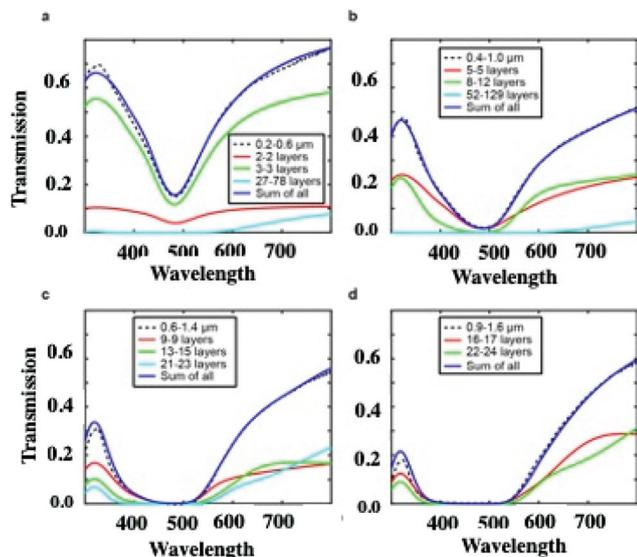
**Fig. 8** Calculated (blue solid traces) and experimental (dashed traces) transmission spectra of 8.2 nm Ag NC supracrystal films with various thicknesses. (a) 0.2–0.6  $\mu\text{m}$ , (b) 0.4–1  $\mu\text{m}$ , (c) 0.6–1.4  $\mu\text{m}$ , and (d) 0.9–1.6  $\mu\text{m}$ . The calculated spectra account for wetting layers with different thicknesses. Colors correspond to different numbers of monolayers.
