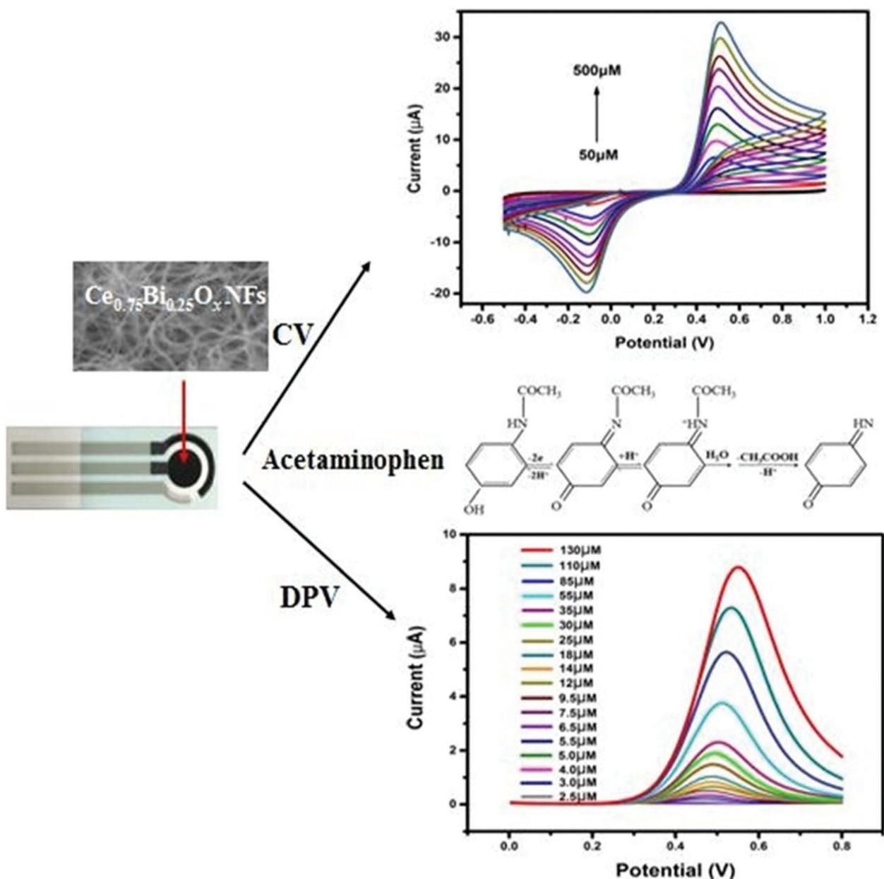
**Fig. 10** Representation of an electrochemical sensor for detecting the pain reliever/fever reducer drug Acetaminophen based on an electrospun CeBiOx nanofibers-modified screen-printed electrode (reprinted with permission from ref. 121. Copyright 2017 Elsevier).
