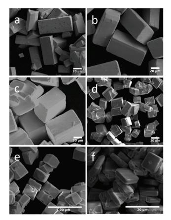
Fig. 7 SEM images of orthorhombic YbFeO<sub>3</sub> with NaOH/KOH mixed mineraliser: (a) 25 M/0 M; (b) 20 M/5 M; (c) 15 M/10 M; (d) 10 M/15 M; (e) 5 M/20 M; and (f) 0 M/25 M. Reproduced with permission from Zhang et al.<sup>170</sup>
