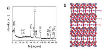
Fig. 17 (a) XRD pattern of sodium iron oxide nanosheets synthesised under microwave irradiation at 180 °C for 5 min. (b) Crystal structure of  $Na_{2.4}Fe_{10.99}O_{16.03}$  viewed perpendicular to the c axis. The pink, red, and grey spheres correspond to Na, O, and Fe atoms, respectively. Reproduced with permission from Wu et al. 328
