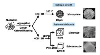
Fig. 5 Crystal morphology control of BiFeO<sub>3</sub> proposed by Li et al. and reproduced with permission. 146
