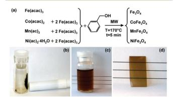
Fig. 19 (a) General reaction scheme displaying the metal oxide precursors employed in the sol-gel synthesis, the solvent, the experimental conditions, and the final composition of the nanoparticles. Photographs of (b) magnetite nanopowder under the influence of a permanent magnet, (c) CoFe<sub>2</sub>O<sub>4</sub> dispersion in ethanol, and (d) CoFe<sub>2</sub>O<sub>4</sub> film on a glass substrate. Reproduced with permission from Bilecka et al. 342
