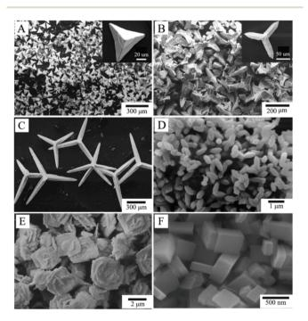
Fig. 4 SEM images of bismuth ferrites prepared by hydrothermal synthesis (A)  $Bi_{12}Fe_{0.63}O_{18.945}$  (pH  $\sim$  12, heating temperature, 180 °C); (B)  $\mbox{Bi}_{12}\mbox{Fe}_{0.63}\mbox{O}_{18.945}\mbox{ (pH}\sim 10,\,180\mbox{ °C); (C)}\mbox{ Bi}_{12}\mbox{Fe}_{0.63}\mbox{O}_{18.945}\mbox{ (pH}\sim 8,\,180\mbox{ °C);}$ (D)  $BiFeO_3$  (200 °C); (E)  $Bi_2Fe_4O_9$  (180 °C); (F)  $Bi_2Fe_4O_9$  (270 °C). Reprinted with permission from Han et al. 145
