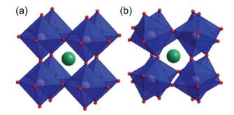
Fig. 2 The ABX<sub>3</sub> perovskite structure (a) view of ideal cubic unit cell with blue [BX<sub>6</sub>] octahedral and green 12-coordinate A sites and (b) the distorted orthorhombic unit cell as found for GdFeO3 where the octahedral are tilted with respect to each other.
