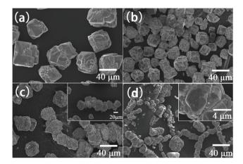
Fig. 6 SEM images of BiFeO<sub>3</sub> obtained by hydrothermal synthesis at 200 °C with 8 M KOH for 6 h in various magnetic fields: (a) 0 T; (b) 4 T; (c) 8 T and (d) 12 T. Reproduced with permission from Hou et al. 151
