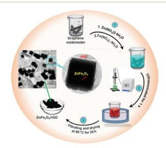
Fig. 13 Reaction scheme for formation of ZnFe<sub>2</sub>O<sub>4</sub>/graphene oxide nanocomposite using sonochemistry. Reproduced with permission from Chen et al. 257
