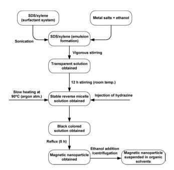
Fig. 15 Flow chart of the typical experimental procedure for the micromulsion synthesis of ferrite nanoparticles (adapted with permission from Mathew et al.). 34 SDS: sodium dodecyl sulphate.
