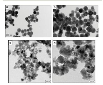
Fig. 12 CoFe<sub>2</sub>O<sub>4</sub> nanospheres (a and b) and nanocubes (c and d) synthesised in water through controlled sonochemistry at room temperature. Reproduced with permission from Abbas et al. 256
