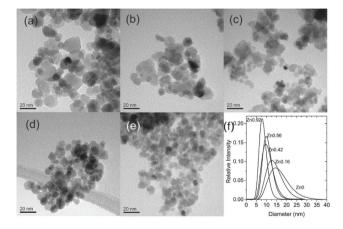
Fig. 21 TEM images showing (a)  $Zn_0$ , (b)  $Zn_{0.16}$ , (c)  $Zn_{0.42}$ , (d)  $Zn_{0.56}$ , (e) Zn<sub>0.92</sub>, and (f) size distributions of all samples prepared through bacterially-assisted synthesis. Data obtained by measurement of n = 200particle diameters per sample. Reproduced from Byrne et al. 351
