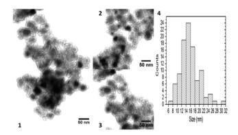
Fig. 14 TEM micrographs and size histogram of Ni<sub>0.4</sub>Cu<sub>0.2</sub>Zn<sub>0.4</sub>Fe<sub>2</sub>O<sub>4</sub> synthesised at T = 90 °C, t = 2 h and for  $P_{diss} = 46.27$  W (1, 2, and 3 represent different areas of the sample; 4 the size histogram). Reproduced with permission from Harzali et al. 266
