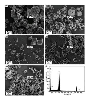
Fig. 20 SEM images of SrTi<sub>1-x</sub>Fe<sub>x</sub>O<sub>3</sub> samples prepared via microwaveassisted hydrothermal method: x = 0.0 (a), 0.05 (b), 0.1 (c), 0.25 (d), 0.4 (e); (f) EDX spectrum of the x = 0.25 sample Reproduced with permission from da Silva et al. 345
