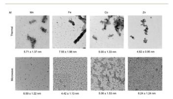
Fig. 18 TEM images of MFe<sub>2</sub>O<sub>4</sub> nanoparticles synthesized by the thermal and microwave synthetic routes. For all the investigated cases, the microwave synthesis produces highly homogeneously dispersed nanoparticles. The numbers below each image display the average nanoparticle size with its deviation. Reproduced with permission from Solano et al. 331
