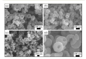
Fig. 11 Scanning electron microscopy images of CoFe<sub>2</sub>O<sub>4</sub> nanospheres prepare via hydrothermal synthesis in the presence of ethylene glycol at reaction times of (a) 6 hours, (b) and (d) 12 hours and (c) 24 hours. Reproduced with permission from Wang et al. 232
