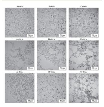
Fig. 9 CoFe<sub>2</sub>O<sub>4</sub> crystallites of three different sizes (A, B and C) coated with oleic acid, citric acid and TiO2. Reproduced with permission from Repko et al. 220
