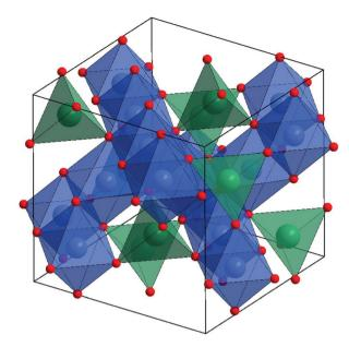
Fig. 1 Crystal structure of normal spinel ferrite ZnFe<sub>2</sub>O<sub>4</sub> highlighting the octahedral Fe (blue) and tetrahedral Zn sites (green) with red oxide anions.
