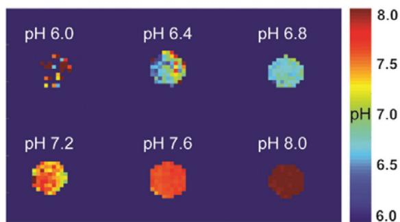
**Fig. 8** CEST MRI on tube phantoms with EuL (3 mM in PBS, RT). pH maps were generated from the ratio of experiments done at  $B_1 = 7.5$  and  $4 \mu\text{T}$ , saturation time 5 s and with the peak at 9.7 ppm.
