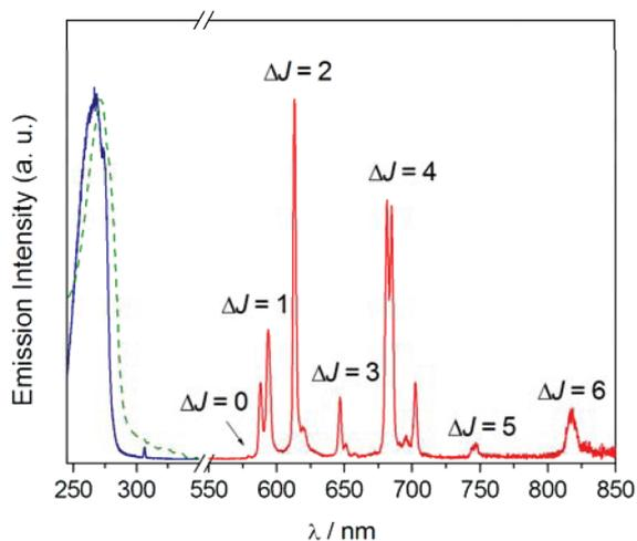
**Fig. 3** UV-Vis absorption (dashed green line), excitation (solid blue line) and emission (solid red line) spectra of EuL recorded in water ( $10^{-5}$  M).  $\lambda_{\text{exc}} = 268$  nm,  $\lambda_{\text{em}} = 613$  nm.
