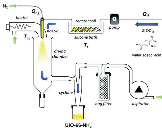
Fig. 6 Schematic illustration of the set-up for the aqueous continuous flow spray-drying synthesis of UiO-66-NH<sub>2</sub>. Reprinted with permission from ref. 58 published by the Royal Society of Chemistry.
