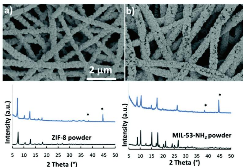
Fig. 17 SEM images and the corresponding XRD patterns of: (a) PAN/ZnO/ZIF-8 and (b) PAN/ $\text{Al}_2\text{O}_3$ /MIL-53- $\text{NH}_2$  composite materials; diffraction peaks of Al-foil are marked with (\*) and diffraction patterns of ZIF-8 and MIL-53- $\text{NH}_2$  reference powder samples are presented for comparison. Reprinted with permission from ref. 172 published by the Royal Society of Chemistry.
