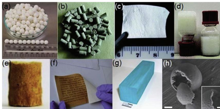
**Fig. 1** Examples showing different shapes of MOFs: (a) granule, (b) pellet, (c) thin film, (d) gel, (e) foam, (f) paper sheet, (g) monolith and (h) hollow structure (scale bar 500 nm (inset 200 nm)). Reprinted with permission from ref. 83. Copyright 2018 Elsevier.
