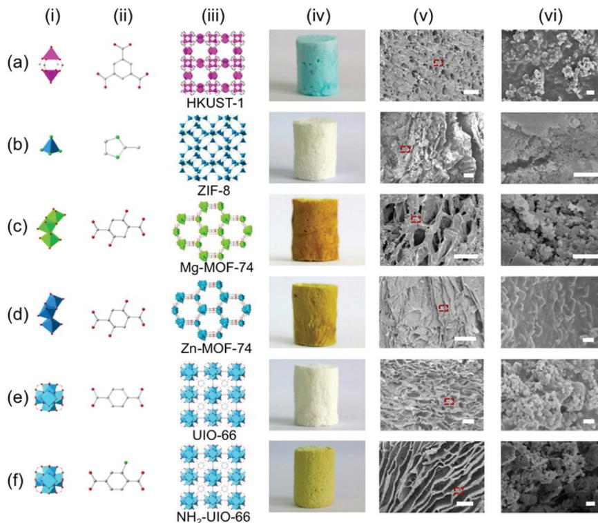
**Fig. 10** The crystal structures of HKUST-1, ZIF-8, Mg-MOF-74, Zn-MOF-74, UiO-66, and NH<sub>2</sub>-UiO-66, and the optical photos and SEM images of the MOF@CMC foams based on these MOFs. The scale bars are 100  $\mu\text{m}$  in v and 1  $\mu\text{m}$  in vi. Reprinted with permission from ref. 133. Copyright 2016 American Chemical Society.
