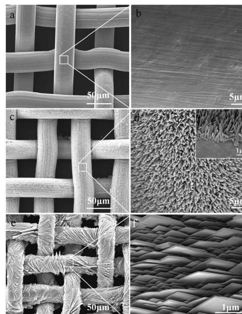
**Fig. 19** SEM images of the bare stainless steel mesh (SSM) (a and b), ZnO nanorods grown on the SSM (c and d) and oriented  $\text{Zn}_2(\text{bIm})_4$  nanosheet grown on the SSM, SSM-500 (e and f). The inset is the cross section of the ZnO rods grown on the SSM. Reprinted with permission from ref. 82. Copyright 2019 Elsevier.
