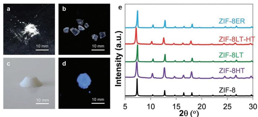
**Fig. 12** (Left) Optical photos of (a) ZIF-8HT; (b) ZIF-8LT; (c) ZIF-8ER and (d) ZIF-8ER samples under 365 nm UV light. (e) PXRD patterns of the different ZIF-8 samples alongside a simulated pattern for ZIF-8. Adapted with permission from ref. 145 published by the Royal Society of Chemistry.
