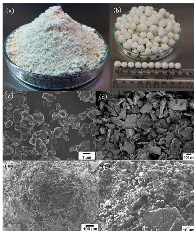
Fig. 3 (a) The optical images of a mixed powder sample of desolvated Zr-MOF (UiO-66) and sucrose (9:1 by weight); (b) optical image of shaped spherical pellets with a diameter around 8 mm; SEM images of the desolvated Zr-MOF (c), the ground sucrose powder (d), and the pellets (e and f). Reprinted with permission from ref. 53. Copyright 2015 Elsevier.
