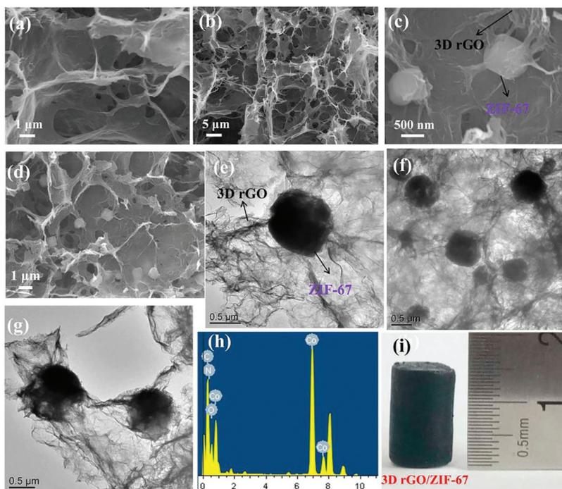
**Fig. 9** The SEM images of (a and b) 3D rGO aerogel and (c and d) 3D rGO/ZIF-67 aerogel, and the TEM (e, f and g), (h) EDX and (i) digital photographs of the 3D rGO/ZIF-67 aerogel. Reprinted with permission from ref. 132. Copyright 2018 Elsevier.
