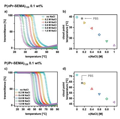
Fig. 5 Influence of the sodium chloride concentration on the cloud point temperature of aqueous (a) P(nPr-SEMA)<sub>130</sub> and (c) P(iPr-SEMA)<sub>128</sub> solutions (0.1 wt%) showing the common observed "salting-out"-effect for thermo-responsive polymers. A linear dependency of the  $T_{cp}$  values on the salt concentration was observed for both polymers (b and d).
