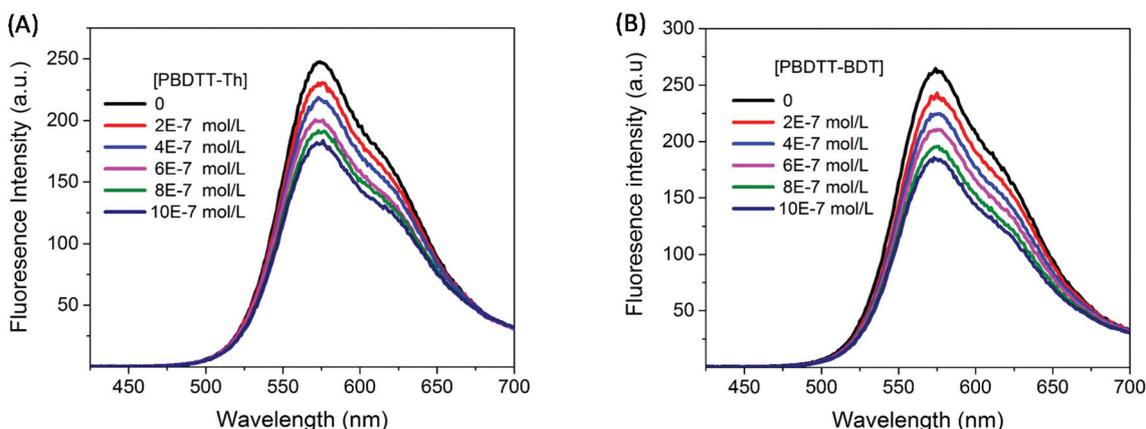
**Fig. 4** Fluorescence spectrum of P3HT ( $4.0 \times 10^{-7}$  M) in chloroform with varying concentrations of the electron acceptor (A) **PBDTT-Th** and (B) **PBDTT-BDT**.
