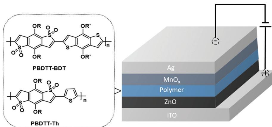
Fig. 1 Device configuration for electron mobility measurements.
