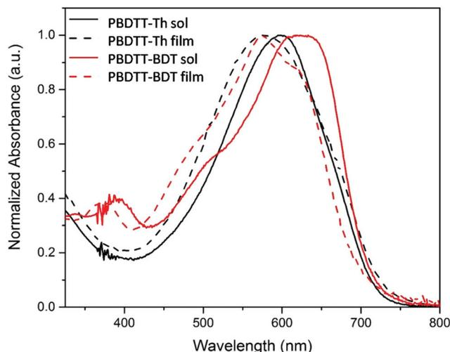
**Fig. 3** Absorption spectra of polymers in solution (CHCl<sub>3</sub>, solid lines) and thin film (cast from CHCl<sub>3</sub>, dashed lines).
