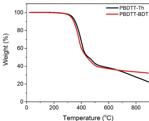
**Fig. 2** TGA curves of **PBDTT-Th** and **PBDTT-BDT**.
