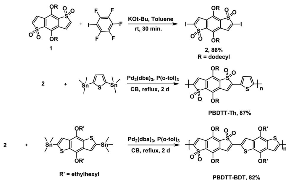
Scheme 1 Synthesis of monomers and polymers.
