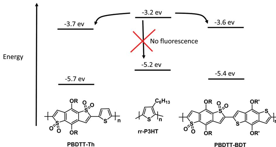
Fig. 5 Illustration of the electron transfer mechanism for fluorescence quenching of rr-P3HT.
