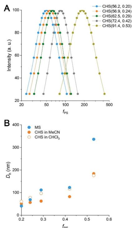
**Fig. 4** (A) Particle size distribution of CHS polymers obtained by DLS measurements in MeCN. (B)  $D_h$  of MS (blue) and CHS (orange) polymers in different solvents. Filled circle: MeCN, open circle:  $\text{CHCl}_3$ .
