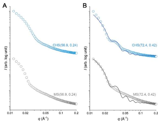
**Fig. 5** Solution SAXS profiles of CHS(56.9, 0.24) (A) and CHS(72.4, 0.42) (B) along with their parent MS. The data were obtained from the MeCN solutions at  $2 \text{ mg mL}^{-1}$  concentration. For the data shown in B, the scattering profiles were fitted with the hard-sphere model.
