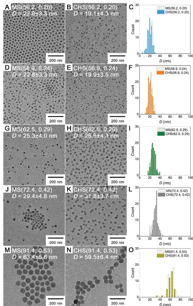
**Fig. 3** TEM images of MS (A, D, G, J and M) and CHS polymers (B, E, H, K and N) cast from the MeCN solution. Size distribution in diameter is shown in C, F, I, L, and O, and the average value is included in the image.
