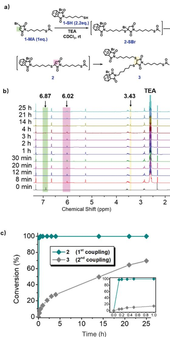
**Fig. 2** (a) The schematic illustration of CTMMC. (b) *In situ* <sup>1</sup>H NMR monitoring of CTMMC (300 MHz, CDCl<sub>3</sub>). (c) The kinetic plot of CTMMC in 1.0 h (inset) and 25 h.
