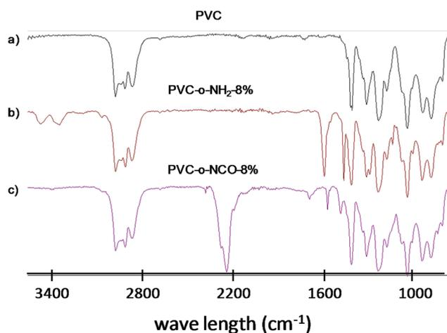
**Fig. 1** FTIR-ATR spectra of (a) pure PVC, (b) PVC-o-NH<sub>2</sub>-8% and (c) PVC-NCO-8%.
