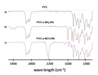
Fig. 1 FTIR-ATR spectra of (a) pure PVC, (b) PVC-o-NH $_2$ -8% and (c) PVC-NCO-8%.
