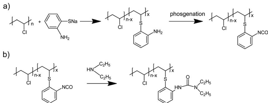
**Scheme 1** a) preparation of aminated PVC (PVC- $\text{o-NH}_2$ -8%) and transformation into PVC bearing isocyanate groups (PVC-NCO-8%), (b) formation of PVC bearing urea groups (PVC-NHCON(C<sub>2</sub>H<sub>5</sub>)<sub>2</sub>-8%).
