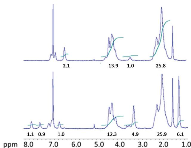
**Fig. 2** H-NMR spectra in CDCl<sub>3</sub> of PVC-o-NH<sub>2</sub>-8% (top) and PVC-NHCON(C<sub>2</sub>H<sub>5</sub>)<sub>2</sub>-8% (bottom).
