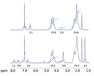
Fig. 2 H-NMR spectra in  $CDCl_3$  of PVC-o-NH<sub>2</sub>-8% (top) and PVC-NHCON( $C_2H_5$ )<sub>2</sub>-8% (bottom).
