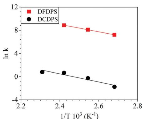
**Fig. 6** Arrhenius plots for the rate constants of polycondensation reactions of DFDPS/BPA (red square) and DCDPS/BPA (black circle) with  $K_2CO_3$  as the base.
