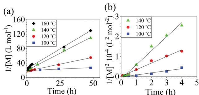
**Fig. 3** Linearized kinetic plots of: (a) second-order reaction for the DCDPS/BPA polycondensation, and (b) third-order reaction for the DFDPS/BPA polycondensation at various temperatures with  $\text{K}_2\text{CO}_3$ .
