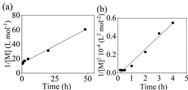
Fig. 4 Linearized kinetic plots of: (a) second-order reaction for the polycondensation of DCDPS/BPA with  $Na_2CO_3$  at 160 °C, and (b) third-order reaction for the polycondensation of DFDPS/BPA with  $Na_2CO_3$  at 140 °C.
