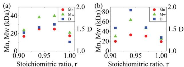
**Fig. 1** The effect of BPA:DXDPS stoichiometry ( $r$ ) on the molecular weight and  $D$  obtained during polycondensation reactions of (a) DCDPS/BPA at 180 °C for 48 h and (b) DFDPS/BPA at 140 °C for 4 h.
