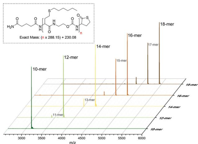
**Fig. 4** MALDI-TOF spectrum of oligomer samples during the synthesis of an *at*-octadecamer in a single continuous run after the 10, 12, 14, 16 and 18<sup>th</sup> reaction cycle. The peaks corresponds to the sodium adduct ( $[M + Na]^+$ ) of the oligomers.
