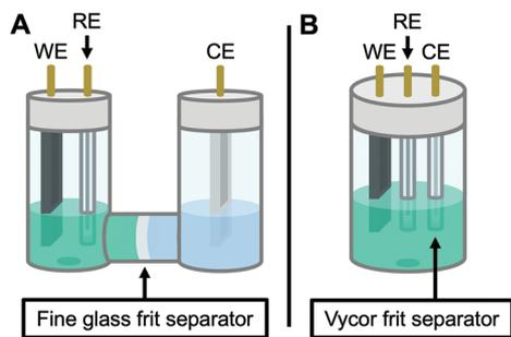
**Fig. 4** Diagram of the apparatus used in this work. Originally, a modified U-cell was employed to separate the working and counter electrode compartments (A). When this separator was found to be ineffective on the time scale of eO-ATRP, a new apparatus was developed using a 5-neck electrochemical flask (see Experimental equipment in ESI†) and vycor frit separators to isolate the counter electrode (B). WE = working electrode, RE = reference electrode, and CE = counter electrode.
