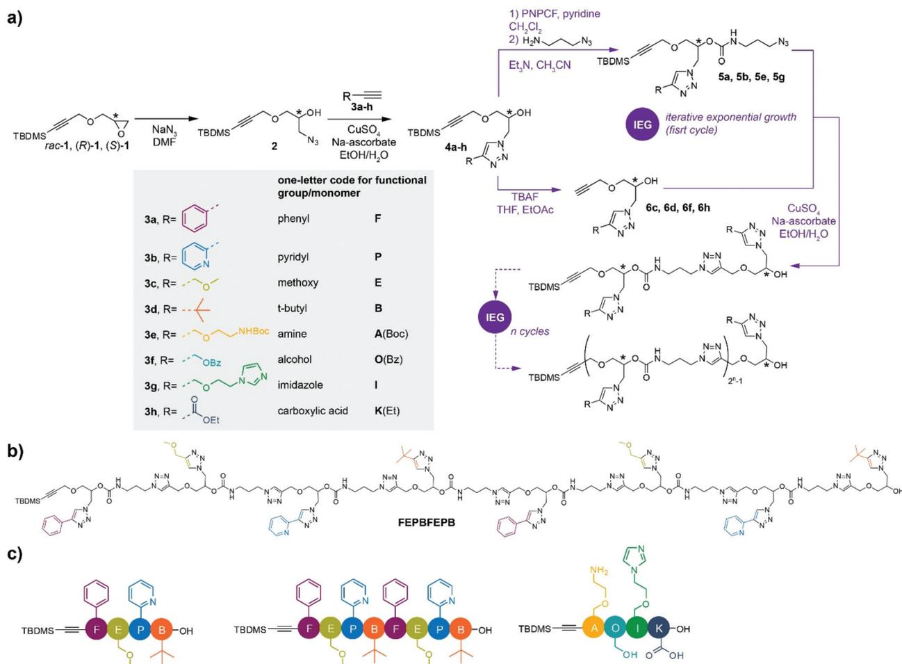
**Scheme 1** . Iterative exponential growth (IEG) strategy to generate discrete multifunctional stereocontrolled sequence-defined oligomers. (a) Synthetic scheme and one-letter code. (b) Structure of octamer FEPBFEPB obtained after 3 IEG cycles. (c) Simplified illustration of the obtained oligomers FEPB, FEPBFEPB and AOIK.
