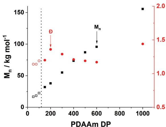
Fig. 9 Evolution of molar mass and dispersity versus PDAAm DP ( $y$ ) for a series of PDMAm<sub>46</sub>-*b*-PDAAm<sub>y</sub> polymers synthesised in the flow reactor with respect to increasing PDAAm DP. The residence time was set to 20 minutes and reactions were performed at either 70 °C (filled) or 90 °C (hollow). Reaction solution were made at 20% w/w total final solids and adjusted to pH 3.
