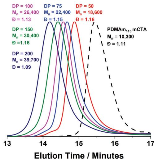
**Fig. 3** DMF GPC chromatograms for a series of PDMAm<sub>113</sub>-*b*-PDAAm<sub>y</sub> block copolymers synthesised in a flow reactor where  $y = 50$  to 200. Polymerisation was conducted at 90 °C, 20% w/w solids and [PDMAm<sub>113</sub>] : [VA-044] = 50 : 1. GPC data was calibrated against a series of ten near-monodisperse poly(methyl methacrylate) standards.
