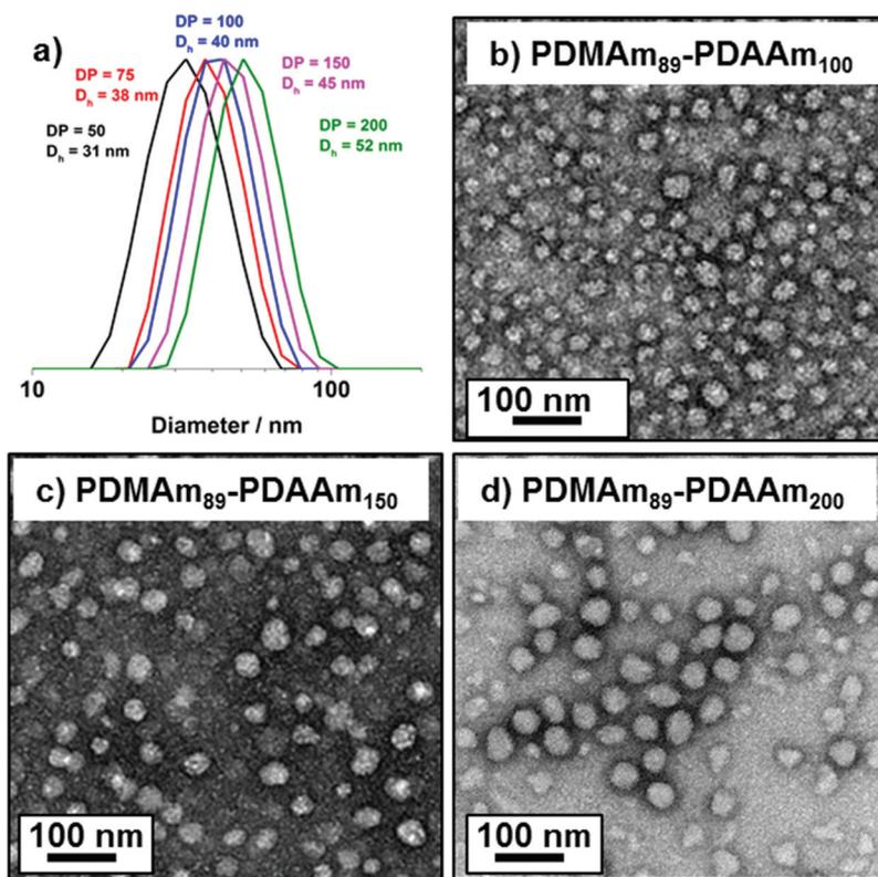
**Fig. 4** (a) DLS traces for PDMAm<sub>113</sub>-*b*-PDAAm<sub>y</sub> polymer nano-objects and representative TEM images for pure sphere morphologies block copolymers where  $y =$  (b) 100, (c) 150, (d) 200. All images were obtained from 0.1% w/w aqueous dispersions of diblock copolymer at pH 3.
