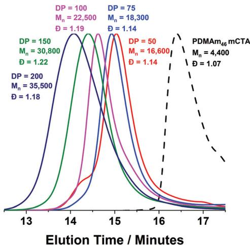
**Fig. 5** DMF GPC chromatograms for a series of PDMA<sub>46</sub>-*b*-PDAA<sub>*y*</sub> polymer nano-objects synthesised in a tubular reactor where *y* = 50 to 200. Reactions were conducted at 90 °C using RAFT aqueous dispersion polymerisation at 20% w/w solids and [PDMA<sub>113</sub>]:[VA-044] = 50:1. GPC data was calibrated against a series of ten near-monodisperse poly (methyl methacrylate) standards.
