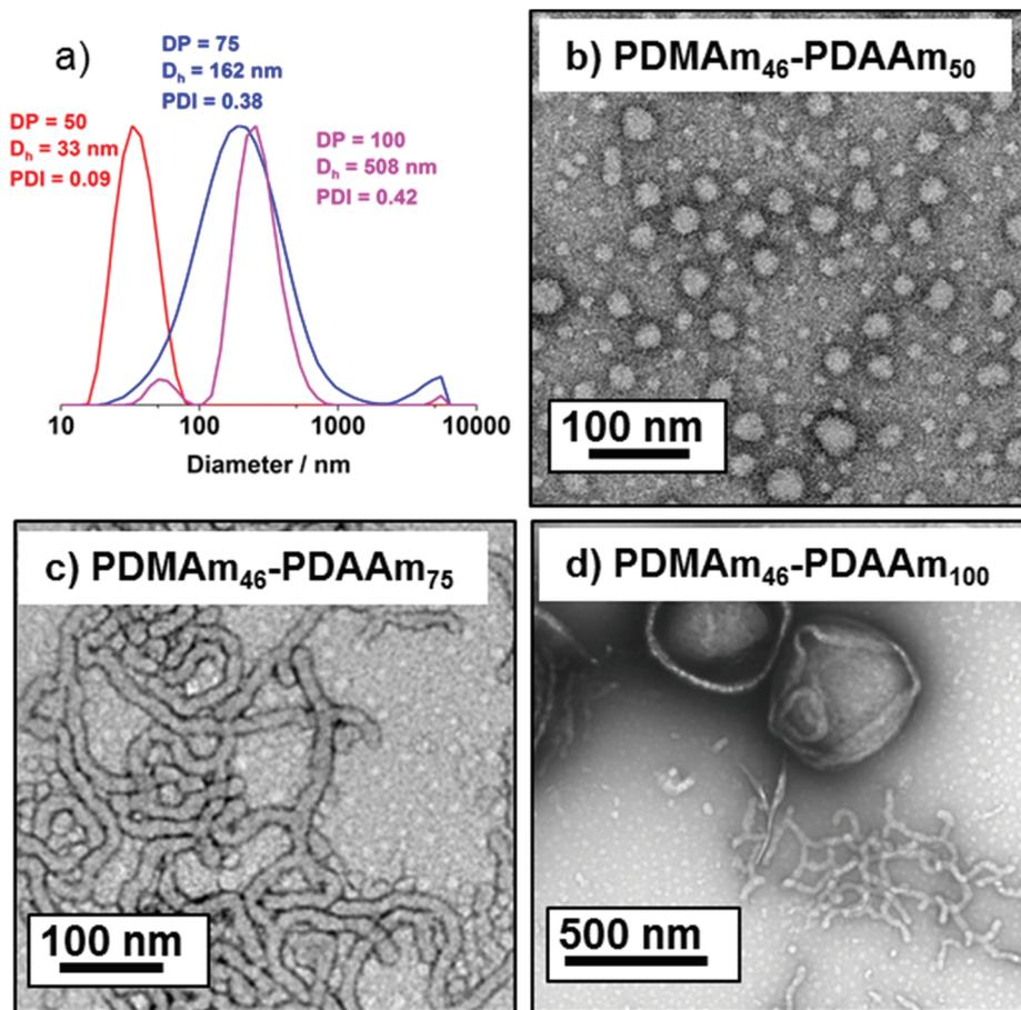
**Fig. 6** (a) DLS traces for PDMA<sub>46</sub>-*b*-PDAA<sub>*y*</sub> polymer nano-objects and representative transmission electron microscopy images for pure sphere morphologies block copolymers where *y* = (b) 50, (c) 75, (d) 100. All images were obtained from 0.1% w/w aqueous dispersions of diblock copolymer at pH 3.
