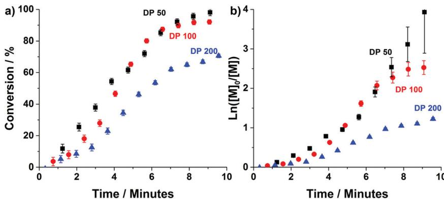
**Fig. 2** (a) Conversion vs. time and (b) semi-logarithmic rate plots for the continuous-flow RAFT aqueous dispersion polymerisation of diacetoneacrylamide (DAAm) using a PDMAM<sub>113</sub> macro-CTA targeting PDAAm DPs of 50, 100 and 200. All reactions were conducted at 90 °C with total solids concentration of 20% w/w and [PDMAM<sub>113</sub>] : [VA-044] = 1 : 0.02.
