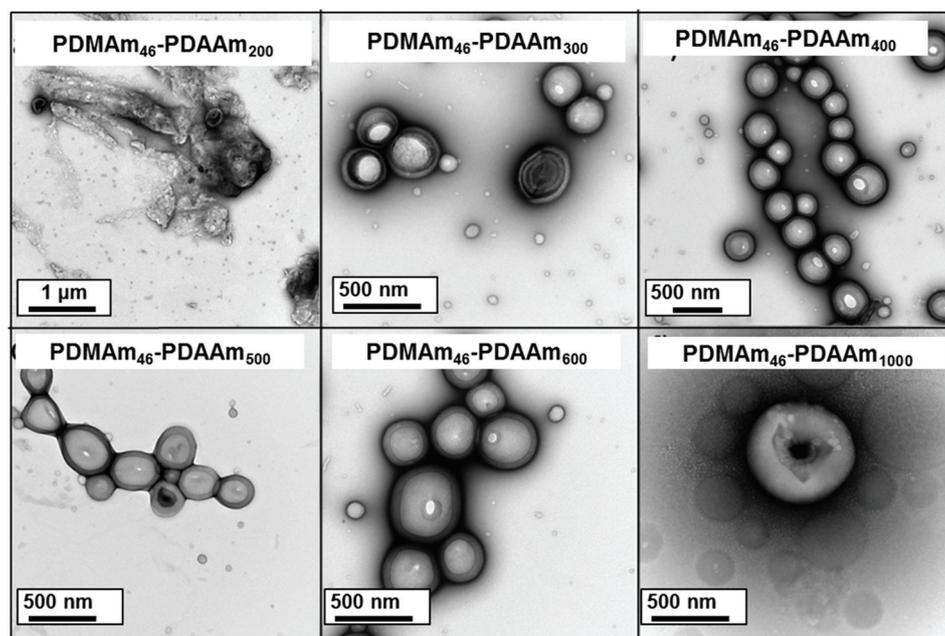
**Fig. 8** Representative transmission electron microscopy images of PDMA<sub>46</sub>-*b*-PDAAm<sub>y</sub> block copolymers, synthesised in the flow reactor, where  $y =$  (a) 200, (b) 300, (c) 400, (d) 500, (e) 600 and (f) 1000. All images were obtained using 0.1% w/w of diblock copolymer at pH 3.
