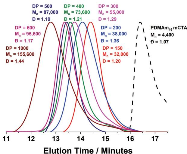
**Fig. 7** DMF GPC chromatograms for a series of PDMA<sub>46</sub>-*b*-PDAAm<sub>y</sub> polymer nano-objects synthesised in a tubular flow reactor where  $y = 150$  to 1000. Polymerisation was conducted at 70 °C using RAFT aqueous dispersion polymerisation at 20% w/w solids and [VA-044] = 0.25 mM. GPC data was calibrated against a series of ten near-mono-disperse poly(methyl methacrylate) standards.
