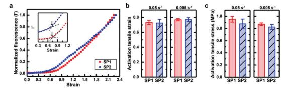
Fig. 8 Activation behaviour of SP1 or SP2 incorporated in PDMS under tension: comparison of (a) the normalized fluorescence intensity as a function of strain at a strain rate of 0.05 s<sup>-1</sup>; (b) the onset of activation strain; (c) the activation stress.<sup>219</sup> Reprinted with permission from ref. 219. Copyright 2018, American Chemical Society.
