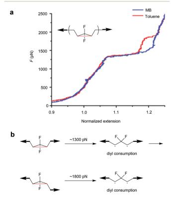
(a) Representative SMFS force curves of Z-gDFC polymer obtained in MB (blue) and toluene (red). (b) The mechanistic scheme for Z-qDFC when the SMFS experiment is performed in toluene. Adapted with permission from ref. 137. Copyright 2016 American Chemical Society.
