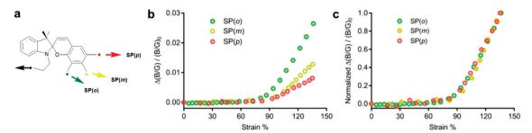
Fig. 9 (a) Spiropyran regioisomers with force handles in *ortho-, meta-* and *para-*position towards the spiro C–O bond. (b) Alteration of B/G intensity. (c) Alteration of B/G intensity normalized to the value at 135% strain.<sup>221</sup> Adapted with permission from ref. 221 Copyright 2018 American Chemical Society.
