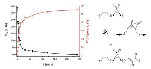
Fig. 4 Ultrasonication of qDCC-PB copolymer leads to ring-opened 2,3-dichloroalkenes (O) with simultaneously decreasing  $M_n$  ( $\blacksquare$ ). Adapted with permission from ref. 120. Copyright 2009 American Chemical Society.
