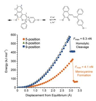
**Fig. 11** 6-Electron electrocyclic ring-opening of NP under mechanical force. (a) Reaction scheme and (b) DFT calculations for three NP regio-isomers. Cleavage of C-O pyran bond is only predicted for the NP with polymer attachment at the 5-position. <sup>226</sup> Adapted with permission from ref. 226. Copyright 2016 American Chemical Society.
