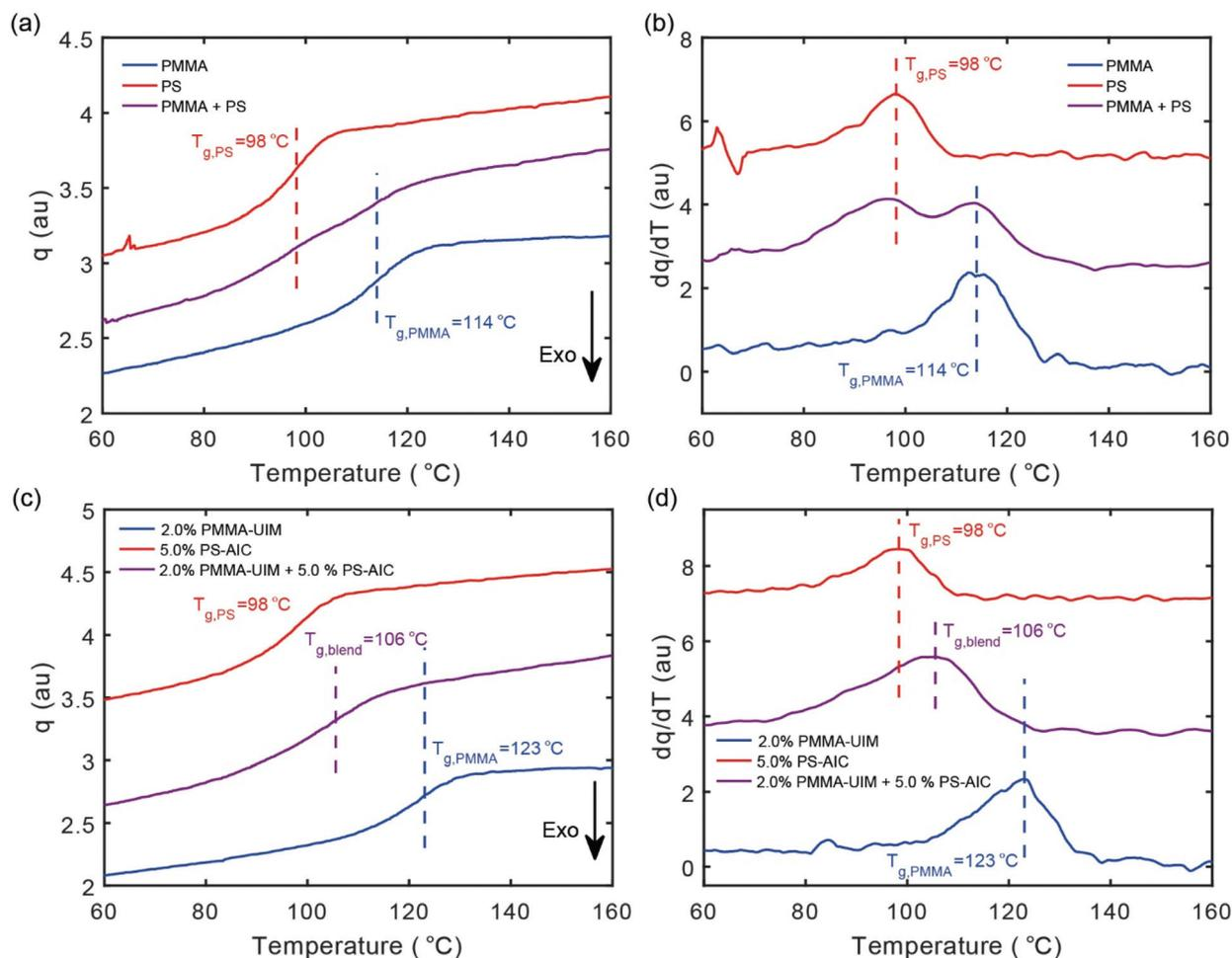
**Fig. 2** DSC thermogram of temperature against (a, c) heat flow and (b, d) first derivative of heat flow on cooling of (a, b) control sample: polymer 10 (PMMA) with polymer 17 (PS) and (c, d) blended sample: PMMA co-polymer 12 (2% PMMA-UIM). PS co-polymer (5.0% PS-AIC) 20 in red, PMMA in blue and blend in purple.
