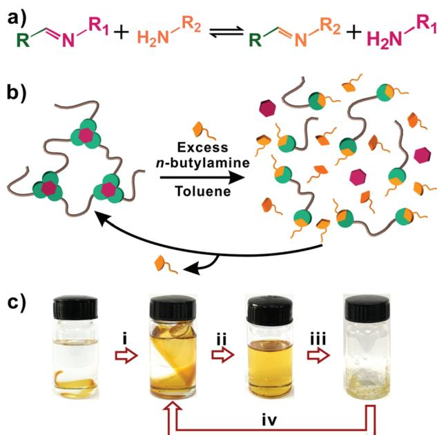
**Fig. 6** (a) Exchange reaction between imine bonds with free amino groups. (b) Schematic diagram of chemical recycling for TAPB using *n*-butylamine. (c) TAPB-0.5 just immersed in toluene (left). (i) TAPB-0.5 was immersed in toluene for 3 days. (ii) *n*-Butylamine was added and the solution was left for another 3 days at room temperature. (iii) The mixture solution was precipitated in methanol and dried. (iv) Conceptual recycling by adding TAA into the degraded product and curing.
