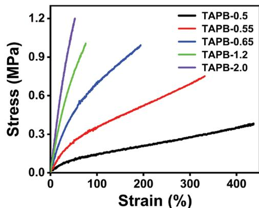
Fig. 3 Typical stress–strain curves of TAPB.
