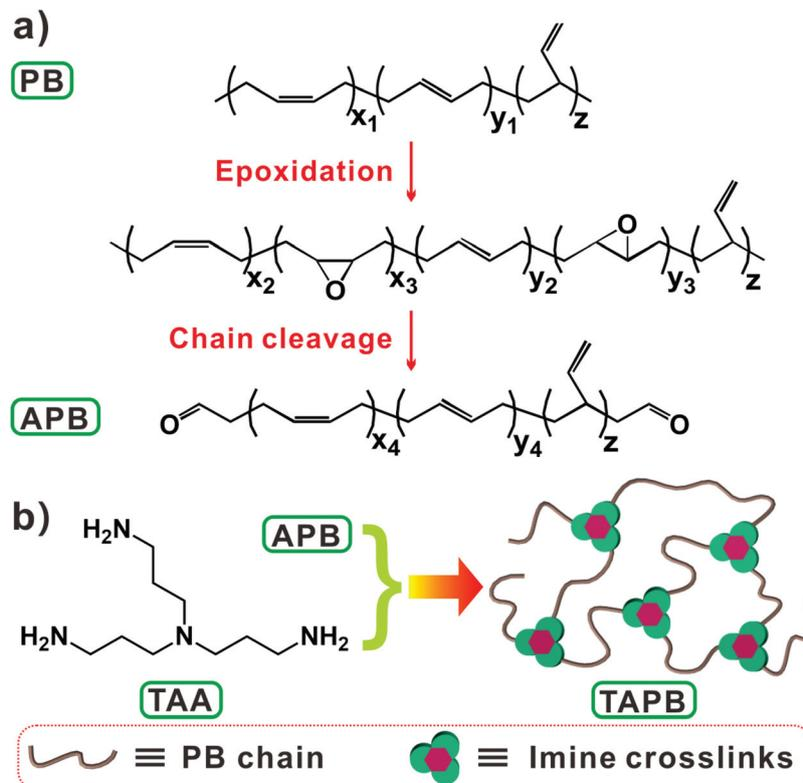
**Scheme 1** (a) One-pot synthesis of APB. (b) Preparation of TAPB by reacting APB with TAA.
