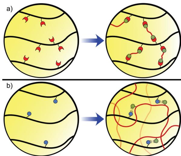
**Fig. 1** (a) Chemical gels are cross-linked by covalent bonds, leading to hydrogels that can resist mechanical strain; (b) physical gels are held together by molecular entanglement and non-covalent forces, resulting in gels with viscoelastic behaviour.
