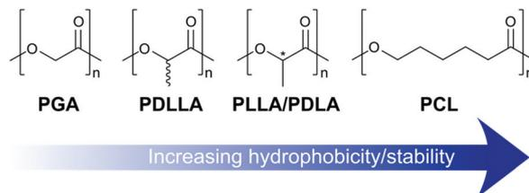
**Fig. 6** Polyester structure dictates the properties of the resulting hydrogel. With increasing hydrophobicity of the carbon backbone, the critical gel concentration decreases, leading to gels that are stable over a wider concentration range. Similarly, the rate of hydrolysis also decreases, due to increased crystallinity. The increased crystallinity of regio-regular PLLA/PDLA vs. PDLLA has a similar effect.
