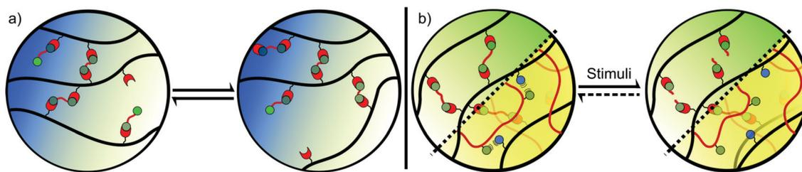
**Fig. 2** (a) Dynamic hydrogels are held together by transiently stable linkages, providing gels with a range of possible properties including self-healing and shear-thinning behaviour; (b) responsive gels undergo a change in properties upon the application of a stimulus. This change may or may not be reversible, and can result from the disruption or formation of both chemical and physical cross-links.
