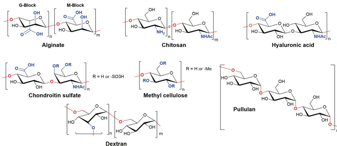
**Fig. 11** Structures of the most commonly used polysaccharides used to form hydrogels for tissue engineering applications. Deviations from the monosaccharide structure of glucose are highlighted in blue, and linkages between monosaccharides in red (s: statistical polymer).
