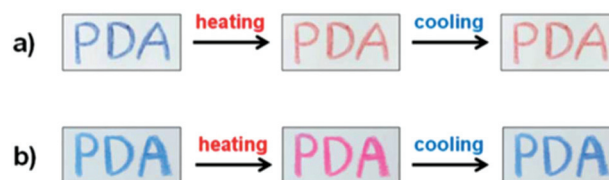
Fig. 22 Handwritten PDA image on paper derived from (a) PDA-wax when heated at 70 °C for 30 seconds then cooled and (b) colorimetric response of PDA-mBzA-wax heated to 120 °C and cooled. Reproduced from ref. 69 with permission from WILEY-VCH Verlag GmbH & Co., copyright [2016].
