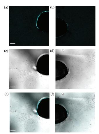
Fig. 7 CLSM images of a rectangular PNIPAAm hydrogel sample swollen to  $d_s = 10\%$  after puncturing with a needle and subsequent compression with tweezers. The images on the left (a, c and e) and the images on the right (b, d and f) compose a whole circular trace of one sample. Fluorescence (a and b); bright field (c and d); overlay (e and f). The scale bar is 100  $\mu m$ . Note how the circular fluorescence trace falls on the needle perimeter.
