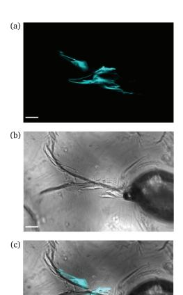
Fig. 8 CLSM images of a rectangular PNIPAAm hydrogel sample swollen to  $d_s$  = 28% after puncturing with a needle and subsequent compression with tweezers. Annotations as in Fig. 6. The scale bar is 100  $\mu$ m. Note how the fluorescence follows the propagation of the crack.
