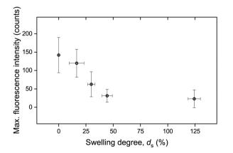
**Fig. 5** Maximum fluorescence intensity as a function of swelling degree. The data have been derived by calculating the mean value and standard deviation stemming from two to five measurements.
