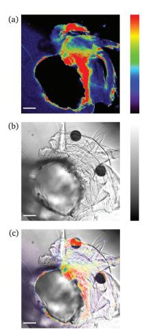
Fig. 6 CLSM images of a needle-punctured PNIPAAm hydrogel sample: (a) fluorescence; (b) bright field; (c) overlay. The intensity values span the 0–255 scale; 0 for black and 255 for red (a); 0 for black and 255 for white (b). The scale bar is 100  $\mu$ m.
