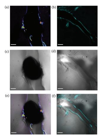
Fig. 9 CLSM images of a rectangular PNIPAAm hydrogel sample swollen to  $d_{\rm s}=36\%$  after puncturing with a needle and subsequent compression with tweezers. The images on the left (a, c and e) and the images on the right (b, d and f) illustrate different regions of the same sample. Annotations as in Fig. 7. The scale bar is 100  $\mu$ m.
