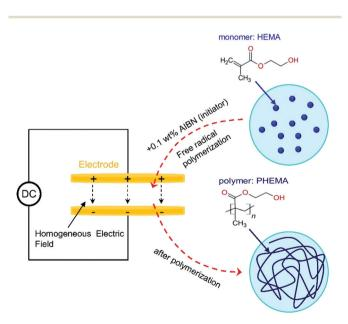
Scheme 1 Sketch of the polymerization experiment using HEMA with a 0.1 wt% AIBN initiator carried out in-between a dielectric sample cell in the absence/presence of a high static electric field. The chemical structures of the HEMA monomer and PHEMA polymer are also shown.
