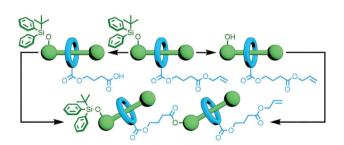
Fig. 9 Orthogonal protecting group strategy towards the iterative synthesis of oligo[n]rotaxanes: the  $^t$ BuPh<sub>2</sub>Si alcohol protecting group can be selectively removed with Bu<sub>4</sub>NF, and the allyl ester can be cleaved with Pd(PPh<sub>3</sub>)<sub>4</sub>. Selective ester formation between the macrocycle of one rotaxane and the axle of another can be ensured in this manner.
