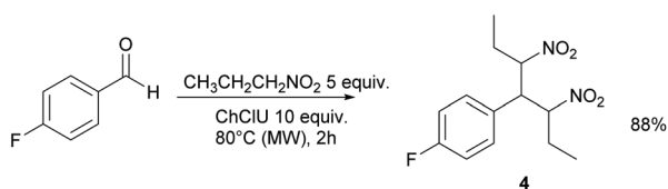
Scheme 2 Reaction between p -fluorobenzaldehyde and nitropropane.
