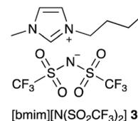
**Fig. 1** The ionic liquid 1-butyl-3-methylimidazolium bis(trifluoromethanesulfonyl)imide ([bmim][N(SO<sub>2</sub>CF<sub>3</sub>)<sub>2</sub>], **3**) used in this study. It should be noted that this anion might also be named as a secondary (sulfonyl)amide.<sup>57</sup> However, imide nomenclature is also reasonable<sup>58</sup> and serves to emphasise the two substituents, along with being consistent with previous work and what is used by the community in, for example, chemical catalogues.
