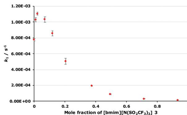
**Fig. 2** The dependence of the unimolecular rate constant ( $k_1$ ) of the reaction of the acetobromogalactose **1** on the mole fraction of [bmim][N(SO<sub>2</sub>CF<sub>3</sub>)<sub>2</sub>] **3** (♦) in methanol at 315 K. Uncertainties reported are the standard deviation of triplicate measurements; some uncertainties fall within the size of the markers used.
