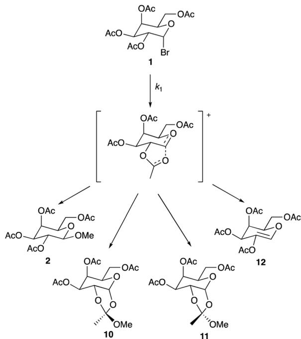
**Scheme 2** The reaction of the galactose **1** with methanol through the proposed intermediate to give the products **2**, **10–12**. The ratio of these products differs when changing the solvent composition.
