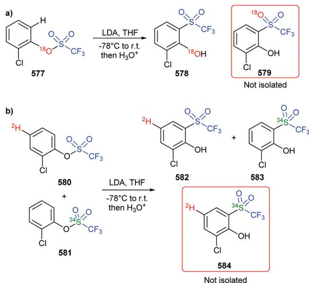
**Scheme 87** (a) <sup>18</sup>O-Scrambling experiment eliminating reversible aryne formation mechanism; (b) crossover experiment indicating an intramolecular sulfonyl migration.
