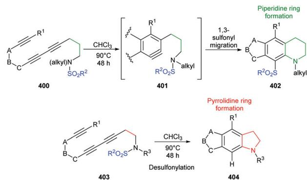
**Scheme 56** Synthesis of tetrahydroquinolines and indolines accompanied by 1,3-sulfonyl migration or desulfonylation via sulfonamide-trapping reactions of thermally generated benzyenes.
