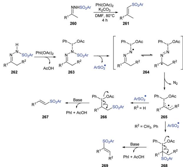
**Scheme 38** PhI(OAc)<sub>2</sub>-mediated synthesis of (*E*)-vinyl sulfones from aliphatic and aromatic *N*-sulfonyl hydrazones.
