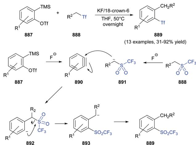
**Scheme 129** Preparation of *ortho*-alkylaryl triflones *via* insertion of C-SO<sub>2</sub>CF<sub>3</sub> bonds into arynes through a tandem nucleophilic attack/intramolecular carbon to carbon 1,3-sulfonyl migration.
